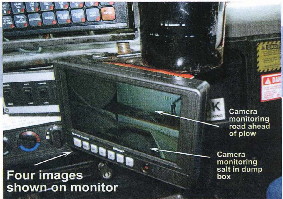
The multiple-blade plow is just one element that is expected to raise the playing field when it comes to winter maintenance. In the cab, operators also use a monitor that shows four different viewpoints of the plow truck.
