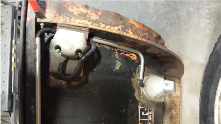
Whelen Lights mounted to a Shop fabricated bracket. These lights also become loose over time. Maybe just a matter of vehicle inspection. Then you cross the line of when is an operator allowed to work as a mechanic. If tightening these lights down is a mechanic's job then the truck is in the shop for repair and not on the road. Should this minor repair be completed by the operator, the truck is still down for a period of time and not in service.
