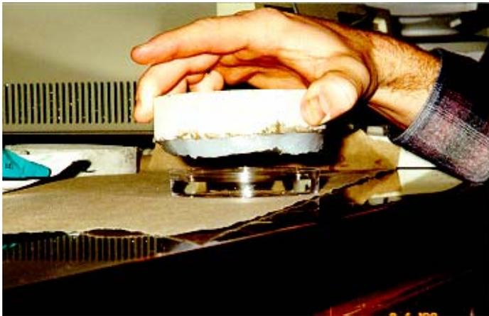
Figure 4-18 Permeability test specimen preparation
