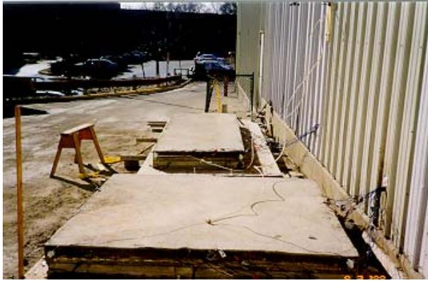
Figure 5-11(b) Slabs connected to power source
