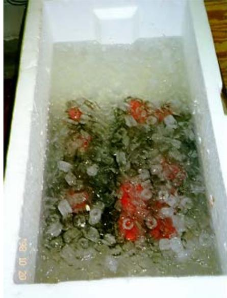
Figure 4-11 Freeze and thaw specimens during taking measurements
