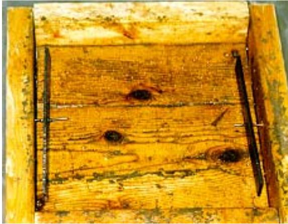
Figure 3-6 Steel plates are used for electrodes
