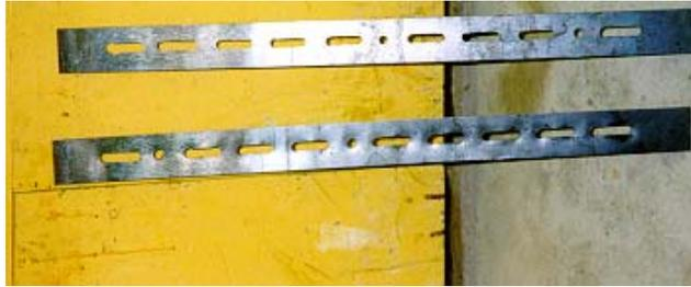
Figure 3-17(a) Steel plate with opening
