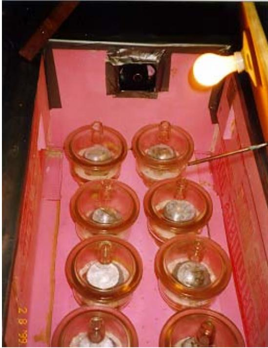
Figure 4-19 Specimens inside moisture-free desiccators
