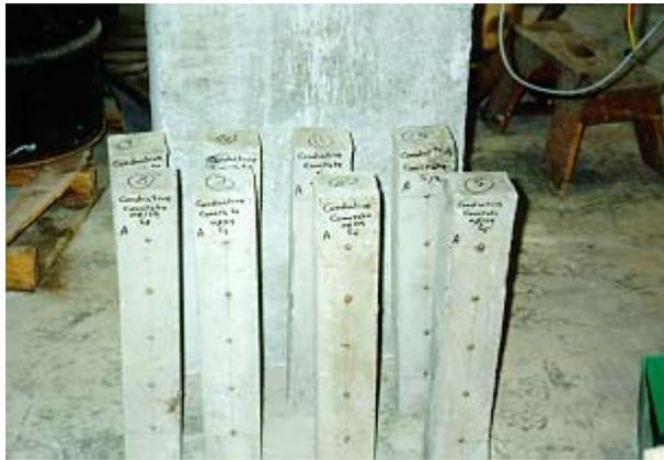
Figure 4-13 Specimens for shrinkage test
