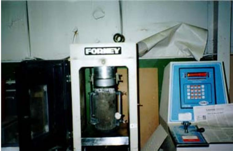
Figure 4-5 Test setup for stress-strain relationship
