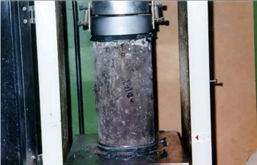
Figure 4-4 Typical failure mode of concrete in compression
