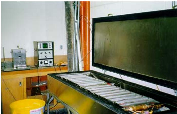
Figure 4-10 Freeze and thaw testing equipment
