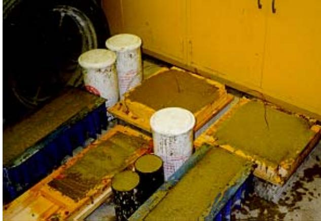
Figure 3-9 Conductive concrete test specimens
