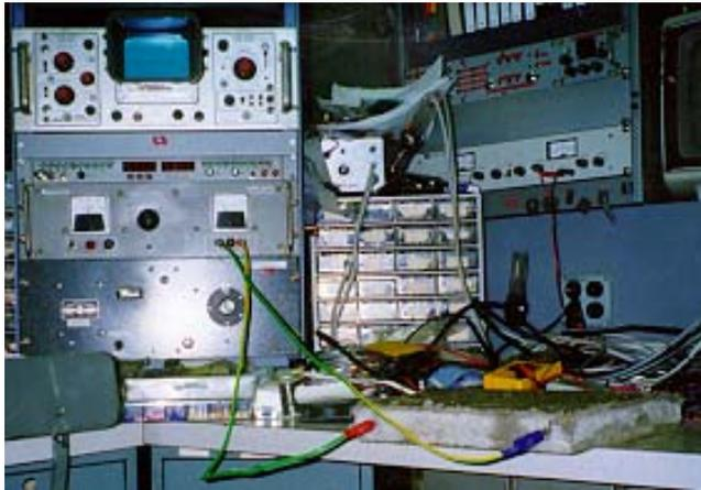
Figure 3-7 Small conductive concrete slab heating test
