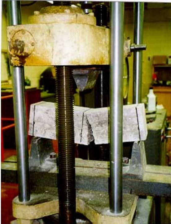
Figure 4-8 Flexural strength – test setup
