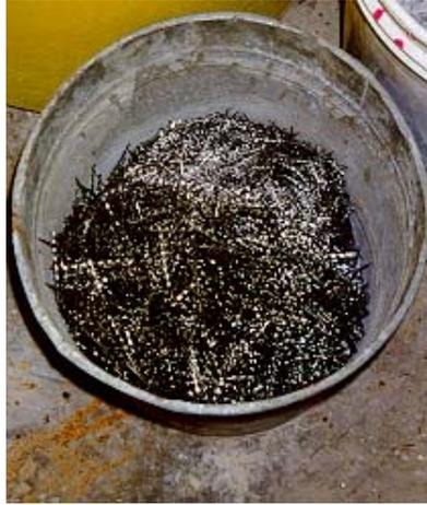
Figure 3-3 Low carbon steel fibers
