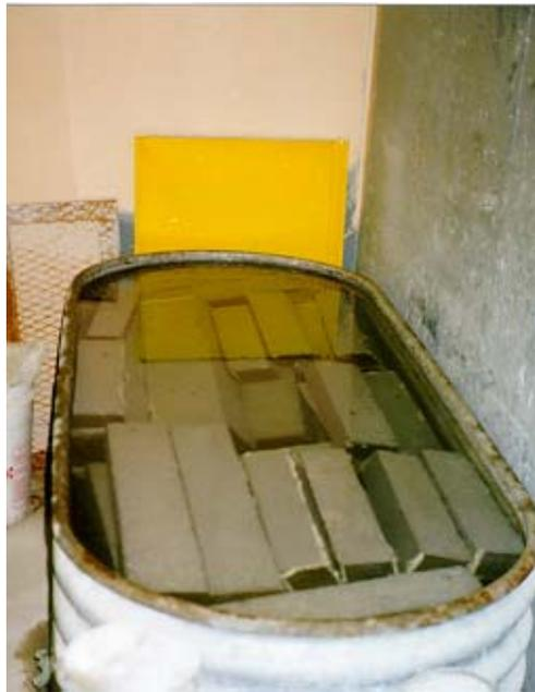
Figure 4-1 Specimens in curing tank
