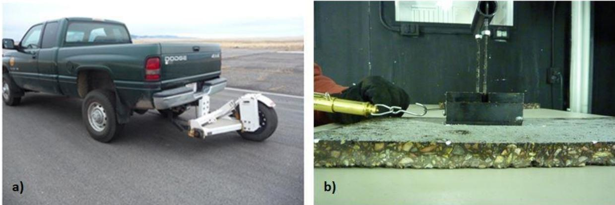
**Figure 35 a) Halliday RT3 Grip Meter, and b) static friction tester.**
