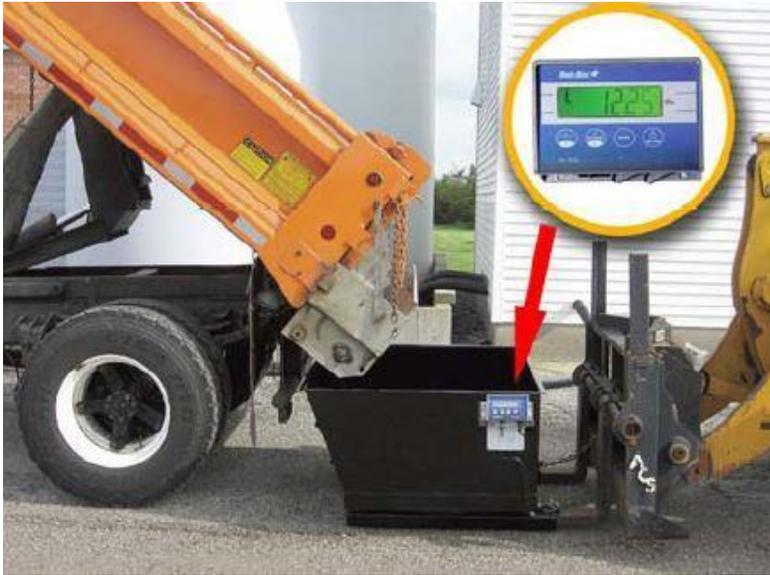
**Figure 28 Spreader calibration (Kimley-Horn, 2010).**
