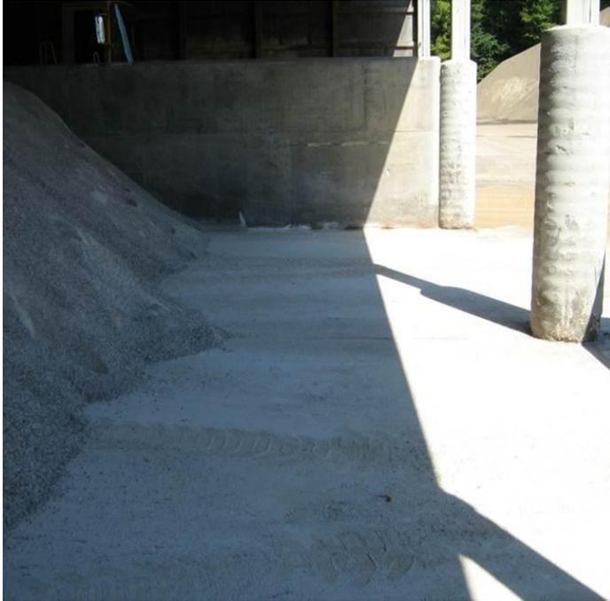
**Figure 98 The 10ft rule. This photo shows how material is kept 10ft back from the door of the storage structure. Photo courtesy of PTC.**
