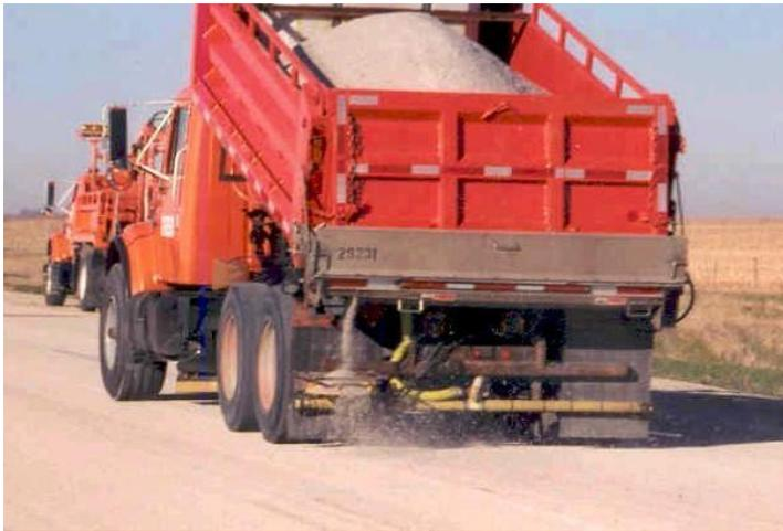
**Figure 21** A conventional tailgate spreader (Nixon, 2009).
