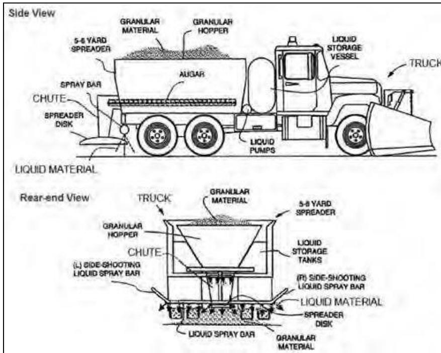
**Figure 24 A system for synchronized application of a plurality of materials (solid or liquid) (Doherty and Kalbfleisch, 2005).**
