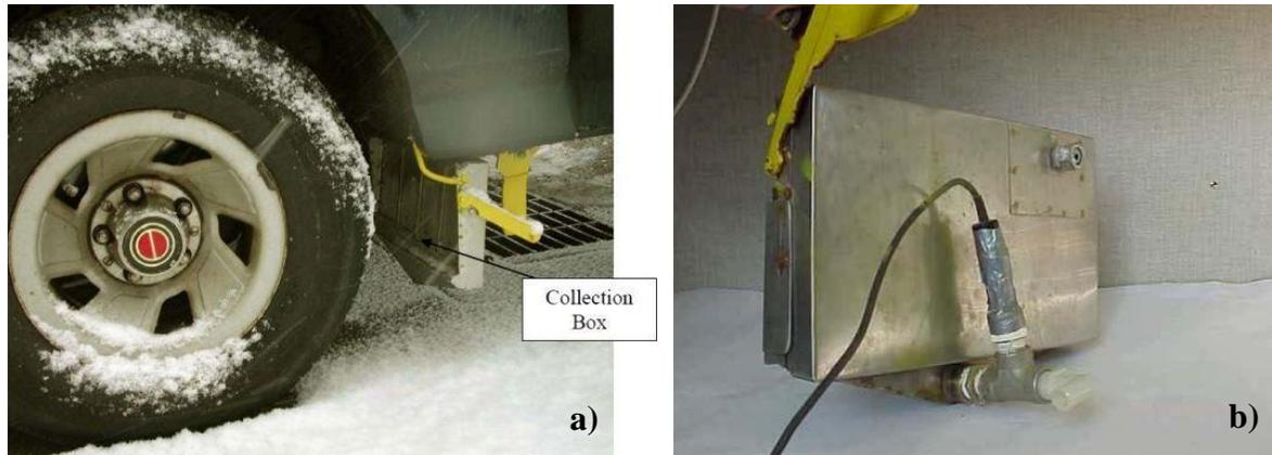
**Figure 37 a) photograph of collection box and b) rear-view collection box with conductivity probe (Garrick et al., 2002a).**
