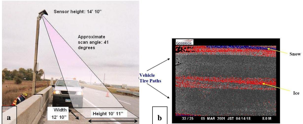
**Figure 42 a) Viewing area and camera position for an LRSS system, and b) a typical picture of a road surface taken by the LRSS (Greenfield, 2008).**
