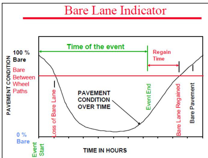
**Figure 3 Derivation of bare pavement regain time (Keranen, 2002).**
