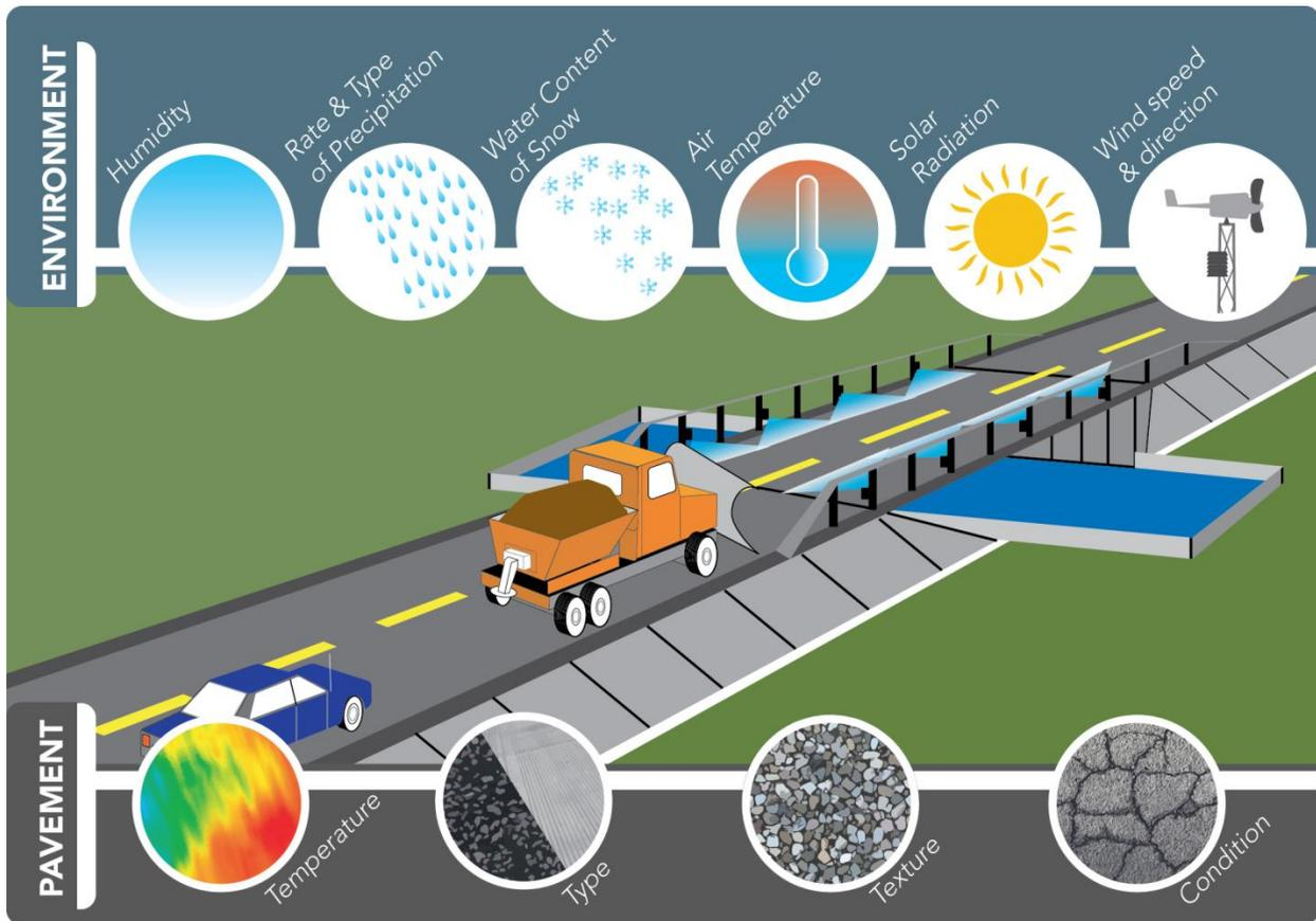
**Figure 31 Environmental conditions and factors that influence pavement conditions and snow and ice control treatments (WTI).**
