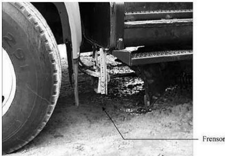
**Figure 39 Frensor device mounted on the highway maintenance concept vehicle (Andrle et al., 2002).**
