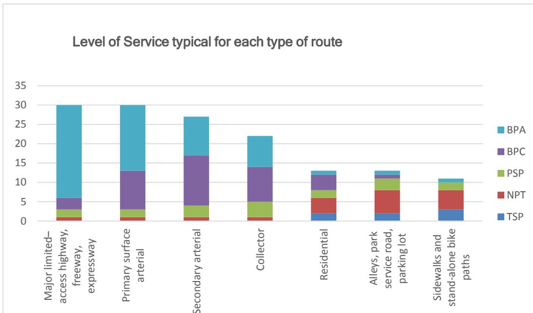
**Figure 8 Level of service for route types based on survey responses. (BPA=bare pavement for all lanes, BPC=bare pavement center of roadway only, PSP=plowed, packed snow, NPT=no plowing or treatment, TSP=trouble spots only treated)**
