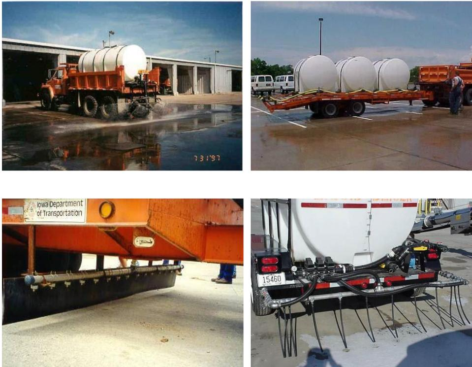
**Figure 25** Examples of anti-icing equipment used by Iowa DOT (Cornwell, 2010).
