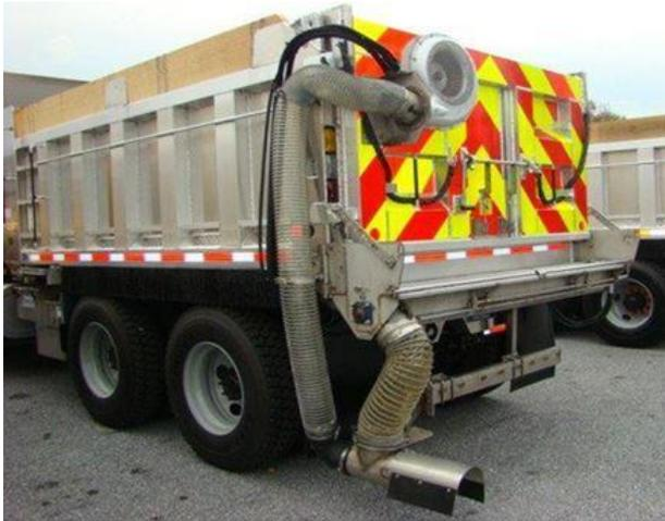
**Figure 27** An example of zero-velocity spreader used by Pennsylvania DOT (Smith, 2014).
