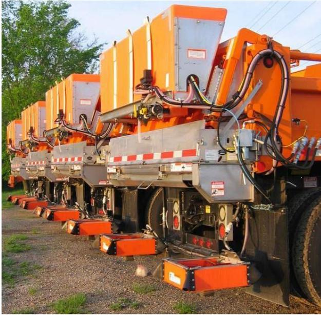
**Figure 22 Iowa DOT tailgate dual augers equipped with a modern pre-wetting system (Burkheimer, 2008).**
