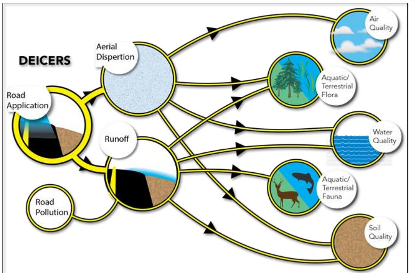
**Figure 11. Pathway of deicer migration into and movement within the environment (adapted from Cheng and Guthrie, 1998).**
