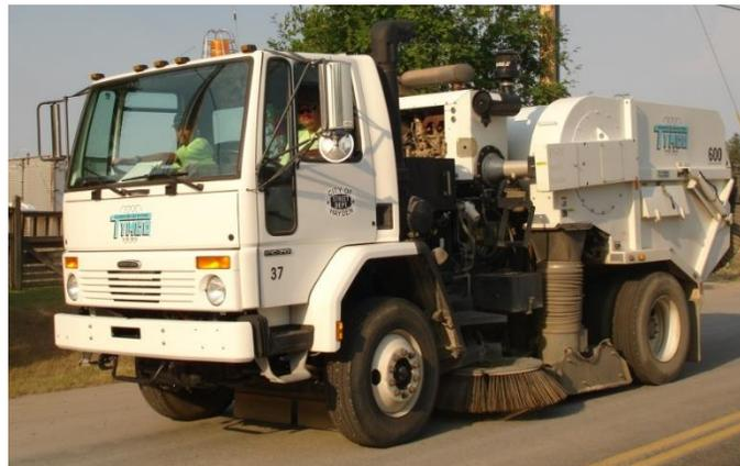
**Figure 43 Picture of a street sweeper with vacuum system ([www.cityofhaydenid.us](http://www.cityofhaydenid.us)).**
