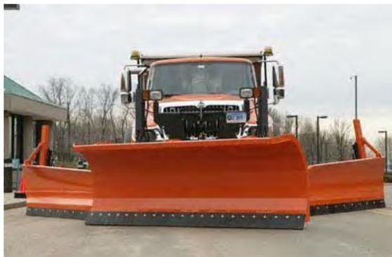
**Figure 14 Photo of a dual wingplow (Rizzo and Moran, 2013).**
