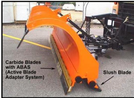
**Figure 13 Prototype snow plow blade design (CTC & Associates LLC, 2010).**
