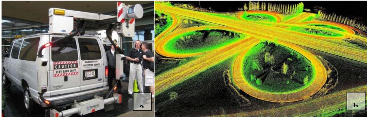
**Figure 41** An example of a) a mobile LIDAR system, and b) an image of a road surface obtained using the LIDAR technique (Yen et al., 2011).
