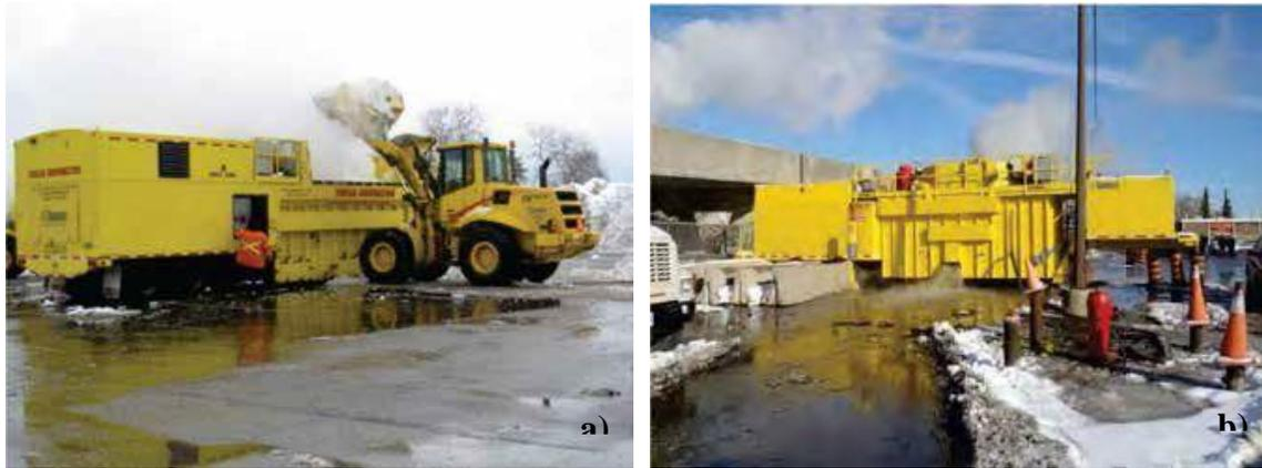
**Figure 20 a) A snow melter in use by the city of Toronto staff during the winter of 2007/2008 and b) another snow melter in use by the city of Toronto staff during the winter of 2010/2011 (Courtesy of City of Toronto, Canada).**
