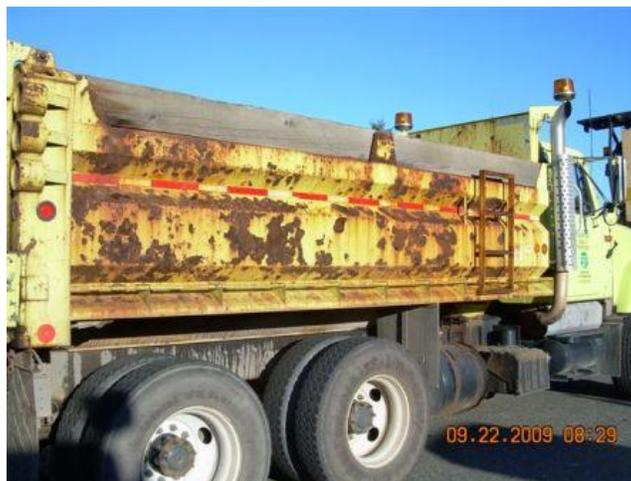
Figure 30 A maintenance vehicle showing extensive corrosion (Mills, 2011).
