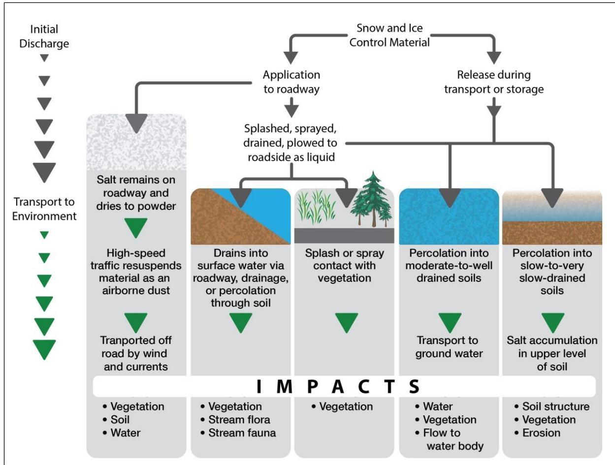
Figure 12. Environmental pathway model modified from Levelton Consultants Limited (2007), showing deicer footprint on the environment.
