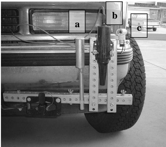
**Figure 38** A surface temperature measurement devices a) Roadwatch™ IR sensors (Ye et al., 2012) b) control products IR sensor, and c) air temperature sensors.
