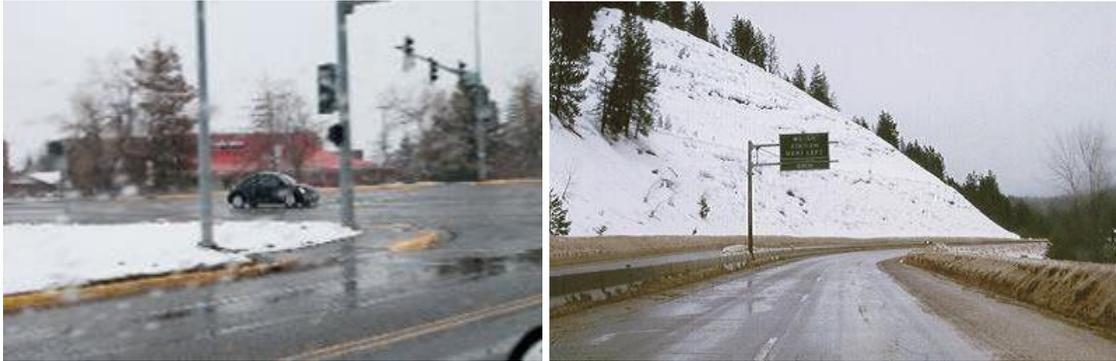
**Figure 4 Examples of “good” road conditions (Veneziano et al., 2014; photos courtesy of WTI and MDT).**
