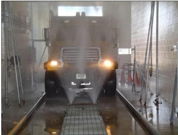
**Figure 29 A tandem axel salt truck being washed off following a salt spreading operation.<sup>2</sup> (Photo courtesy of the City of Toronto).**
