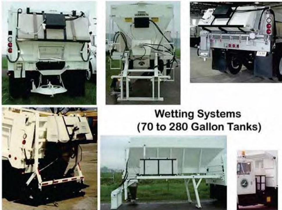
**Figure 23 Pre-wetting equipment used by the Ohio DOT (Ohio DOT, 2011).**
