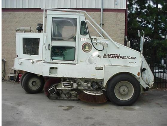
**Figure 44 Picture of mechanical broom street sweeper (www.sweepers.com).**
