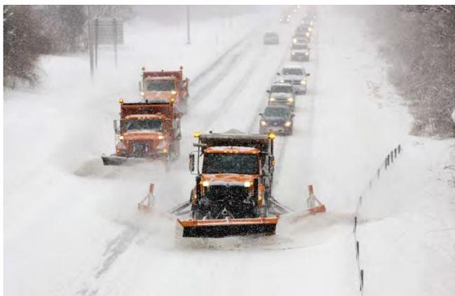
**Figure 17 Tandem plowing technique (Rizzo and Moran, 2013).**
