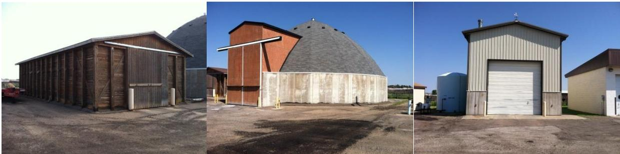
**Figure 96 Typical storage buildings used by the Kansas DOT; (left) 1960-70's wood frame, (middle) dome with barn doors, (right) newer construction of a wash bay facility. Photos courtesy of Kansas DOT.**
