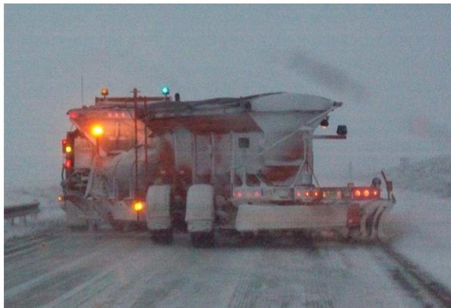
**Figure 16 Picture of a tow plow from the back (Anderle, 2013).**
