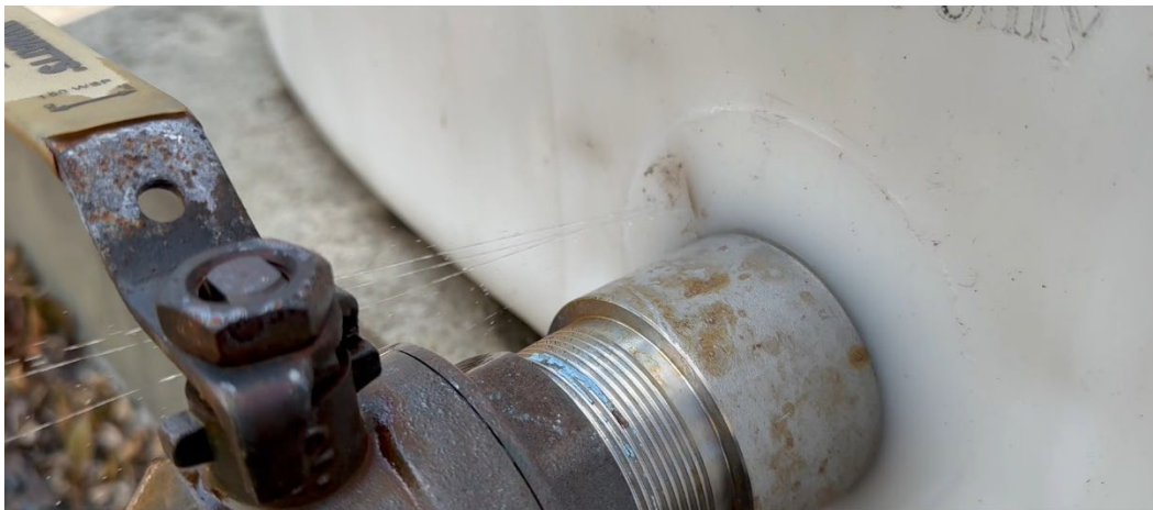
Figure 18. Pinhole Leak on Poly Tank (Source: Massachusetts DOT)
