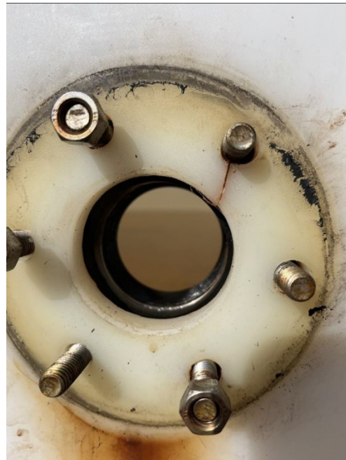
Figure 17. Poly Tank Split at Flange (Source: Massachusetts DOT)
