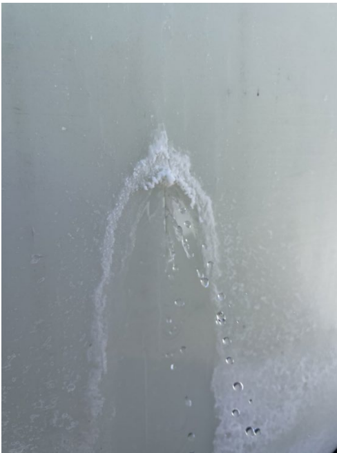
Figure 16. Poly Storage Tank Crack Leaking Deicer (Source: Maine DOT)
