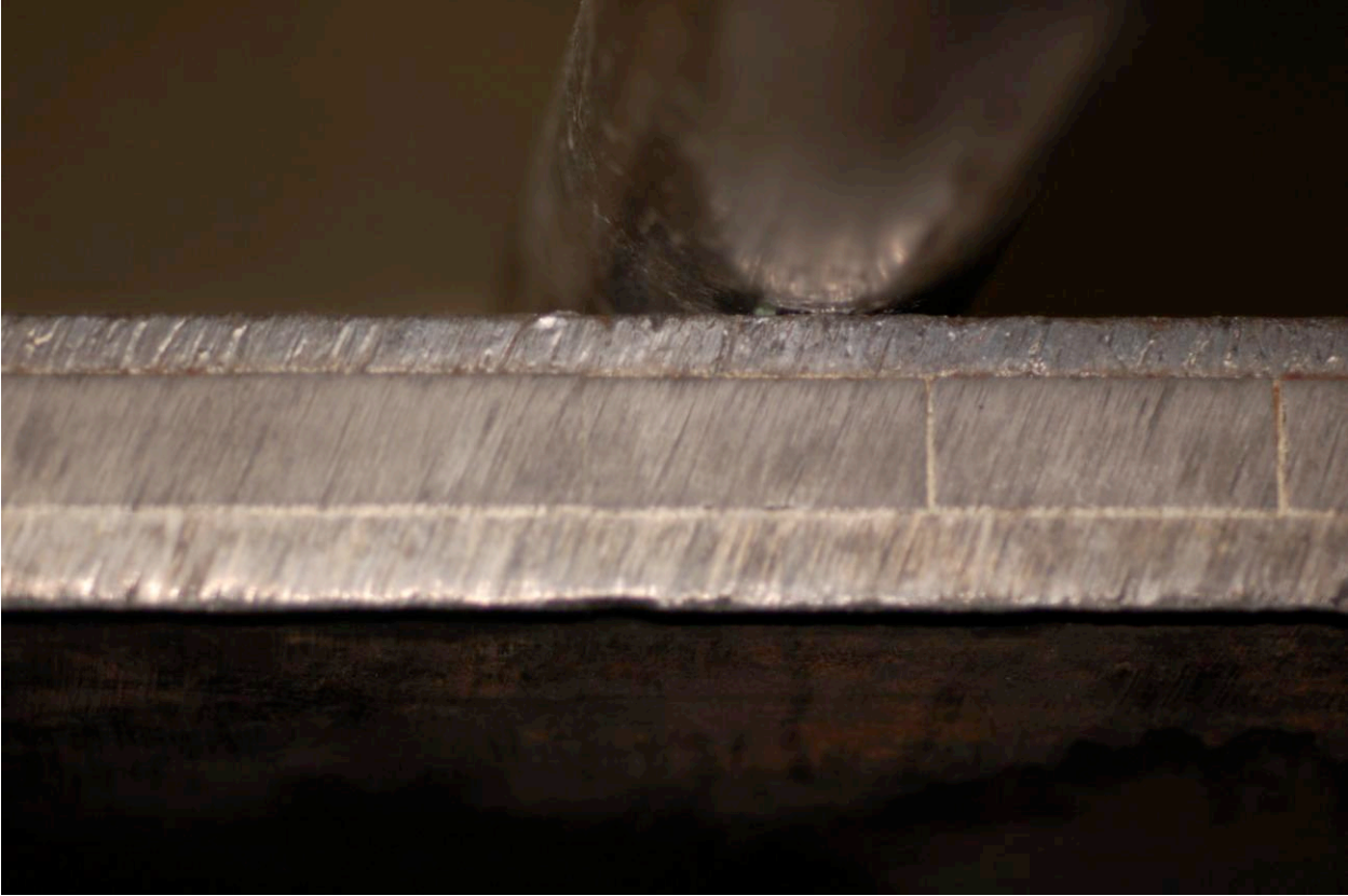
Figure 2.7 Field Tested Blade from Supplier M (no cracks or chips)
