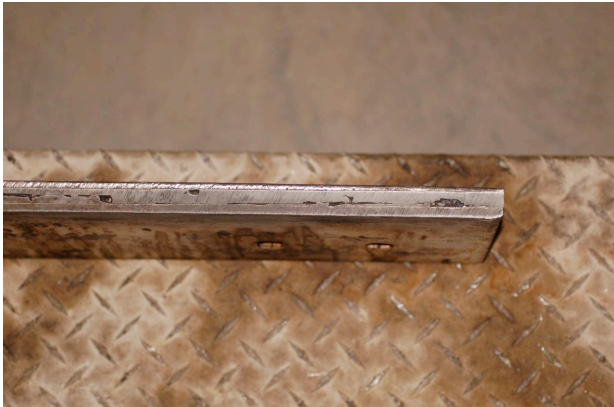
Figure 2.6 Field Tested Blade from Supplier V (cracked and chipped)
