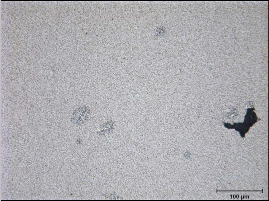
Figure 2.2 Supplier E, Polished, Magnification 200X Showing Voids and Void Clusters
