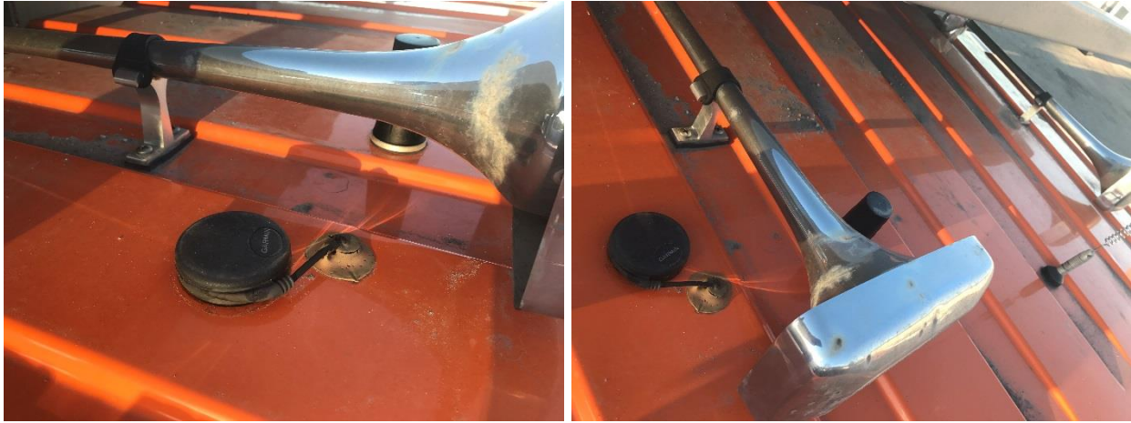
Figure 6. Zonar AVL/GPS System Antennae Locations
