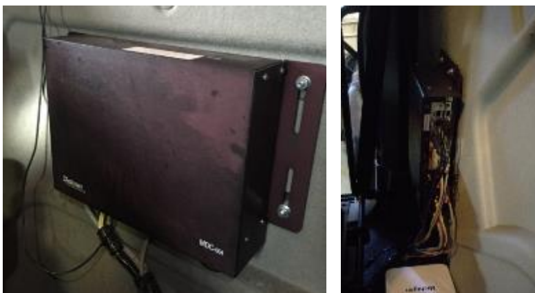
Figure 20. AVL Hardware Installation: Connector Panel Facing Down (right) and Connector Panel Facing Sideway (left)
