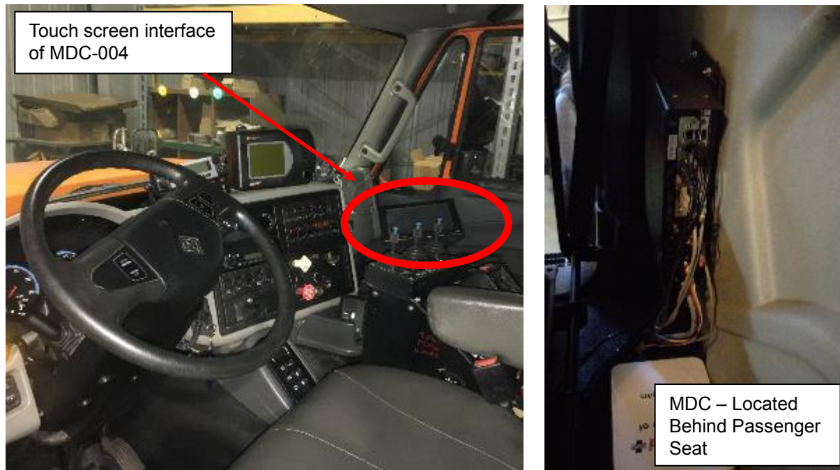
Figure 4. Location of Parsons AVL Hardware in MDOT Snow Plow
