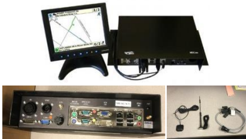
Figure 3. Mobile Data Computer (MDC) and AVL Hardware (above) and Back View of MDC, Antennae and Cable (below)
