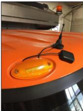
Figure 21. Improper Installation of Cellular/GPS Antenna Cables
