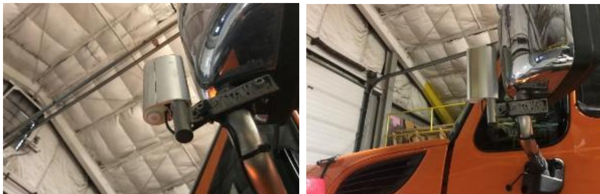
Figure 7. RoadWatch Pavement Temperature Sensors on MDOT Snow Plow Vehicle
