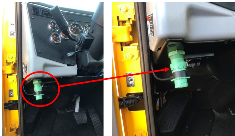
Figure 10. Location of NDOT Snow Plow Vehicle Diagnostic Connection with AVL/GPS System
