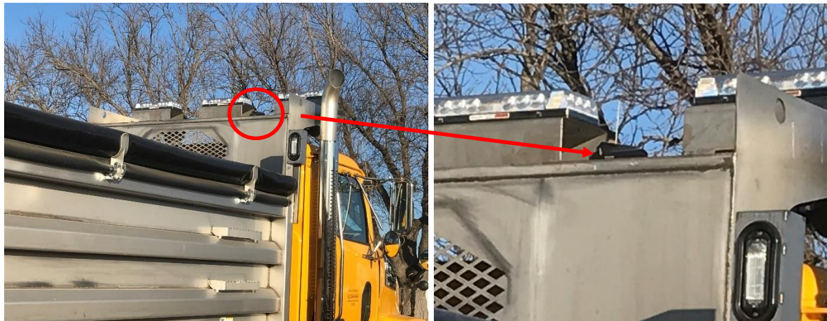
Figure 9. Location of NDOT AVL/GPS System Antennae on Snow Plow Vehicle
