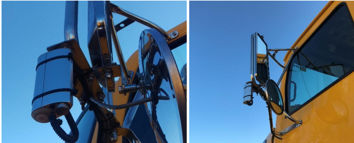
Figure 7. NDOT RoadWatch Air / Pavement Temperature Sensor Location on Plows
