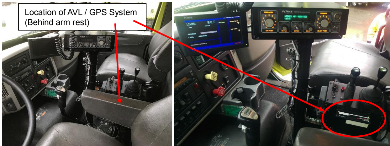
Figure 4. WSDOT Snow Plow Equipment and Location of LT6 AVL/GPS System
