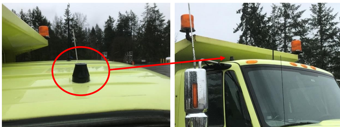
Figure 11. WSDOT Dual GPS / Cellular Antenna Location on Vehicle Roof
