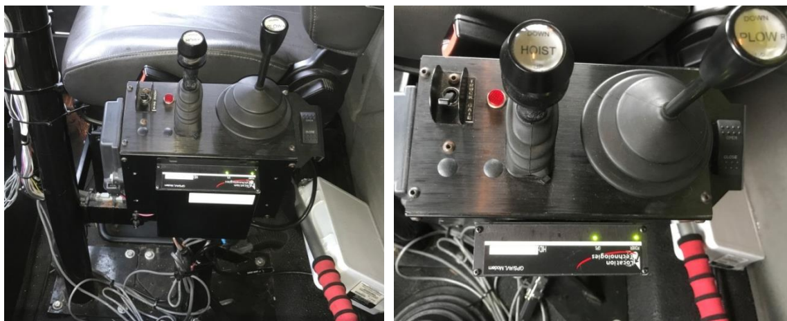
Figure 5. LT6 AVL/GPS System Mounting Location
