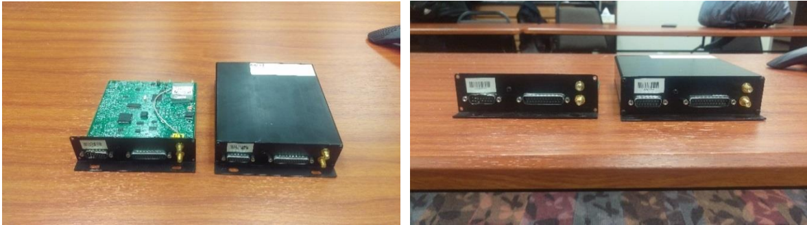
Figure 3. WSDOT AVL/GPS System Hardware Units (Un-covered and Covered)
