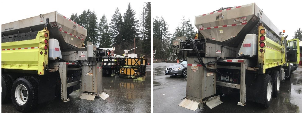
Figure 9. WSDOT Snow Plow Spreader Equipment and Spray Tank
