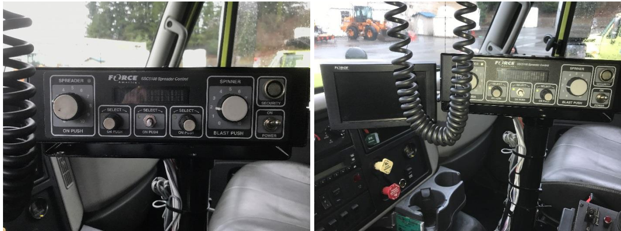
Figure 6. WSDOT Spreader Controller Equipment and Screen
