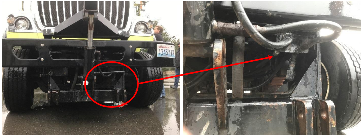
Figure 8. WSDOT Snow Plow Hydraulic Sensor Location
