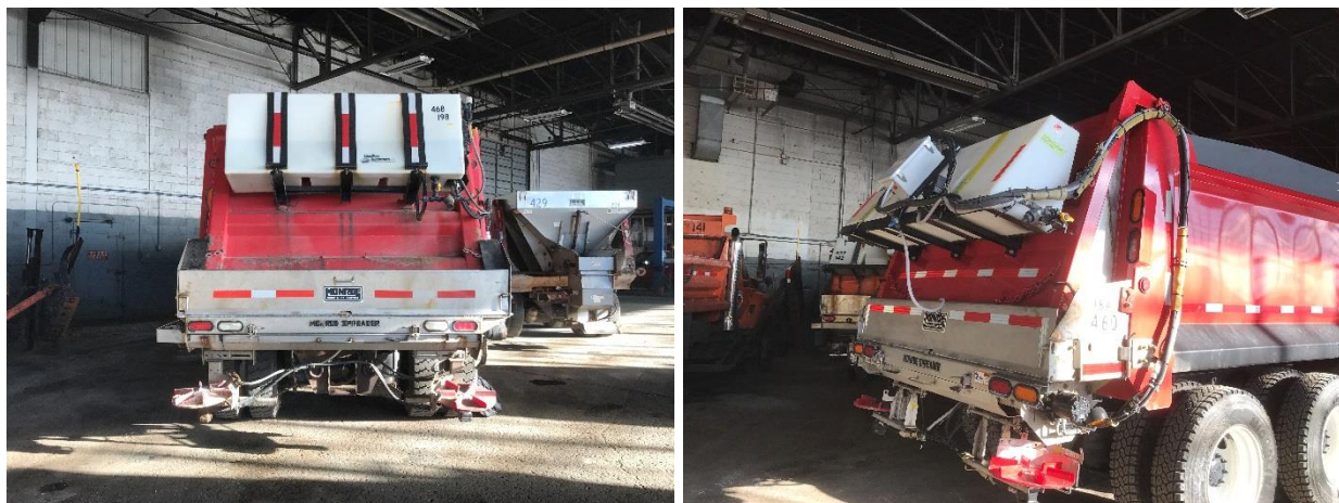
Figure 8. Sauk County Snow Plow Spreader Equipment and Spray Tank
