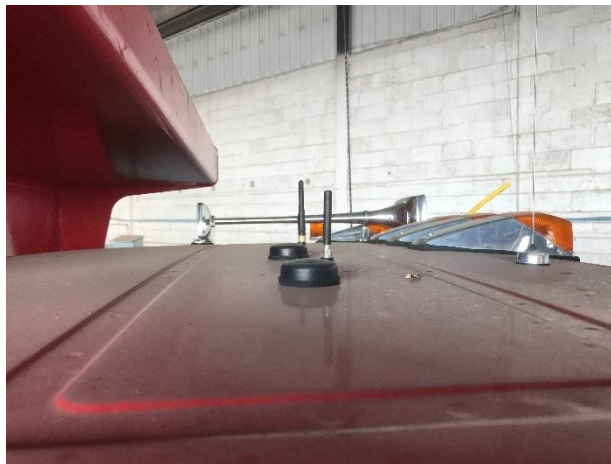
Figure 3. PreCise AVL/GPS System Antennae for Cellular and GPS / Wi-Fi Connection
