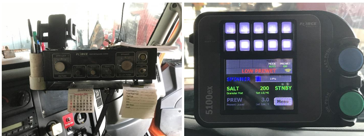
Figure 5. Sauk County Spreader Controller Types (5100 right and 5100EX left)
