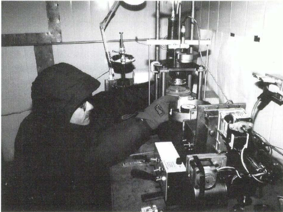
Figure 7 Direct simple-shear apparatus (from Schweizer, 1998)
