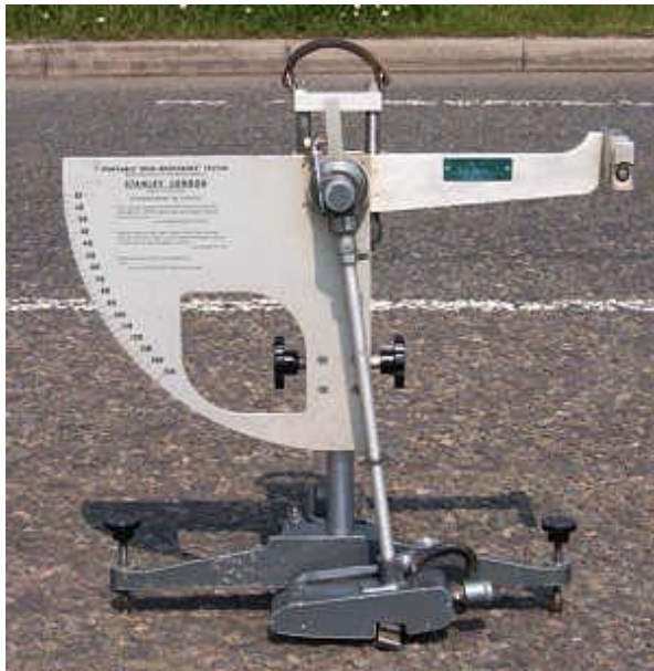
Figure 11 British Pendulum Tester (picture from http://www.highwaysmaintenance.com/skidtext.htm )
