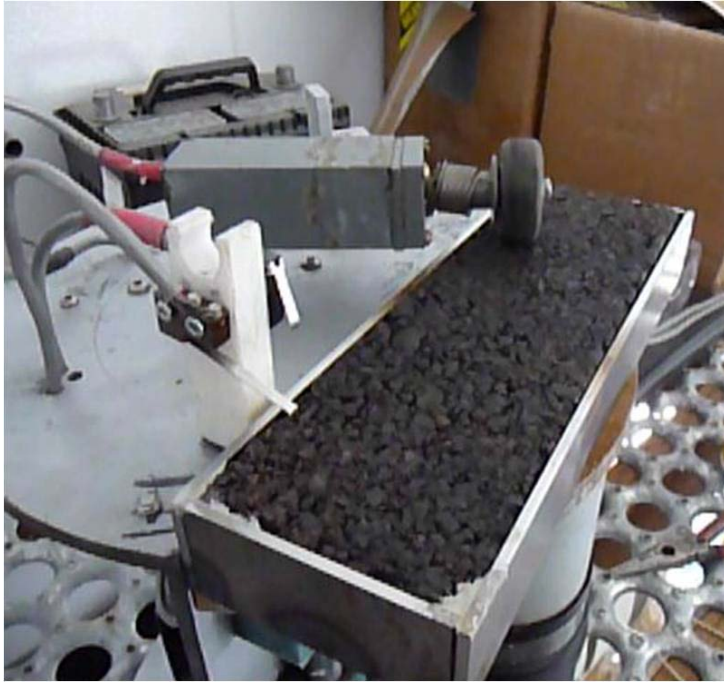
Figure 10 In Road Friction Sensor measuring friction on a 3 in x 9 in asphalt pavement sample
