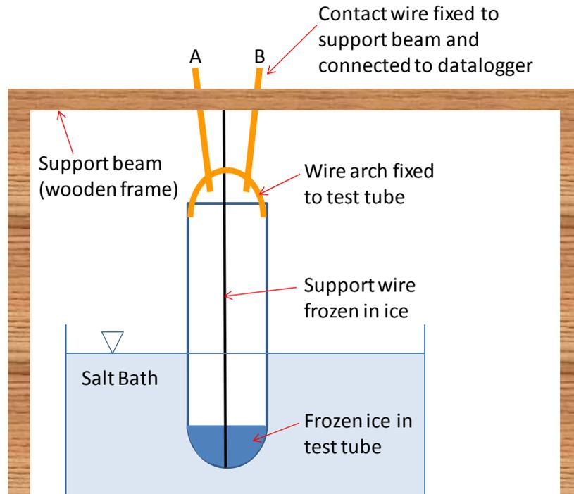
**Figure 15. Mauritis Ice Undercutting Apparatus**
