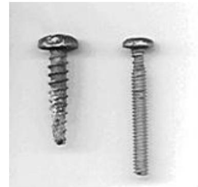
***Filiform corrosion*** is a special form of crevice corrosion which happens beneath some types of coatings.
