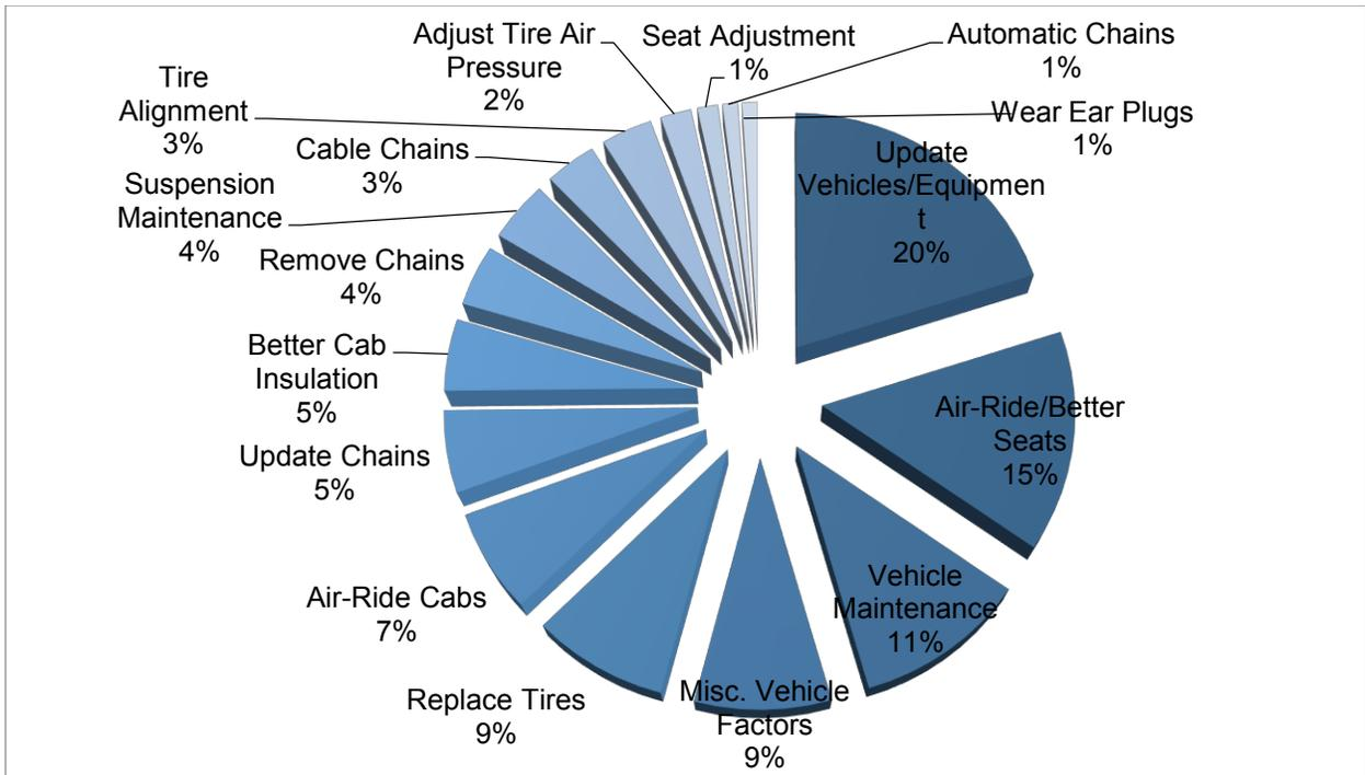
**Figure 132. Vehicle-related Ways to Eliminate Vibration**
