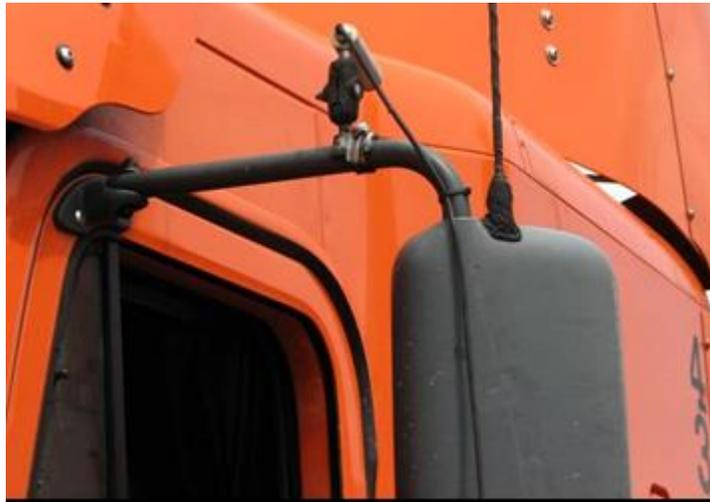
**Figure 6. Example of the Backwards-facing Side Camera Mounted on the Outside Rearview Mirror**
