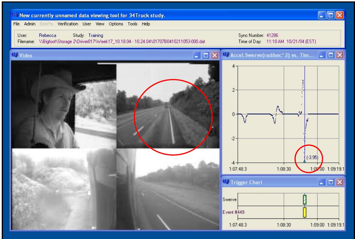
Invalid: In this example, the swerve value (**Gyro Rate**) has gone above the trigger threshold value of 2 degrees/sec<sup>2</sup> to 3.68 degrees/sec<sup>2</sup>. Looking at the video, it can be seen that the driver is only changing lanes into a turn lane and it not swerving to avoid a conflict.
