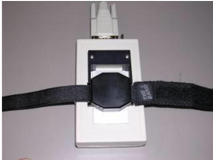
**Figure 10. Downloading Data from Actigraph Device**
