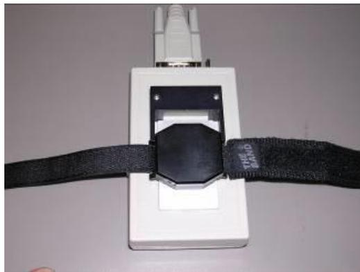
**Figure 52. Proper Actigraph Watch Interface Placement for Downloading Data**
