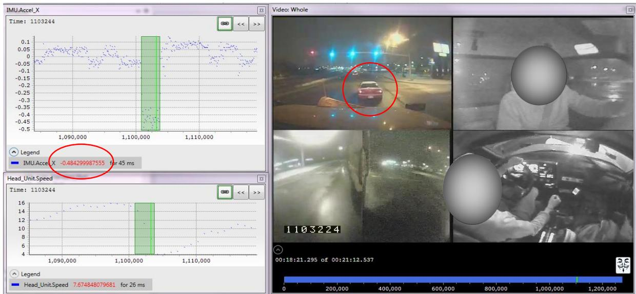
**Figure 13. Example of a Validated Trigger where the Longitudinal Acceleration was of Greater Magnitude than the Pre-set Value of  $|0.20\text{ g}|$**
