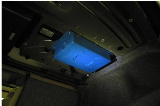
**Figure 4. The Main DAS Unit Installed behind the Driver's Seat**
