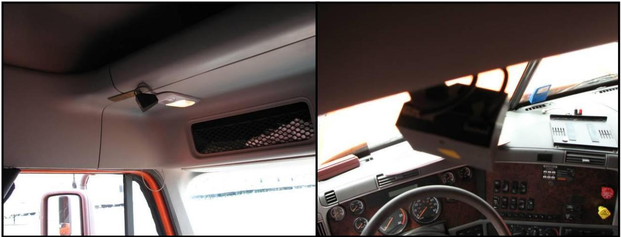
**Figure 7. Example of the Dome Camera Mounted on Roof of Cab (left) and View from Behind the Dome Camera (right) providing an Over-the-shoulder View of the Driver, Steering wheel, and Dashboard**
