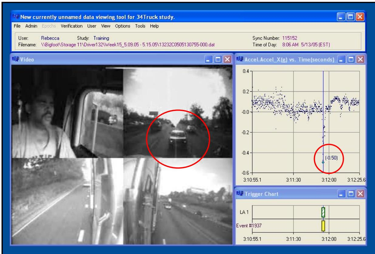
Invalid: In this example, the Accel\_X value has dropped below the trigger threshold of -0.35g to -0.37g. Looking at the video, it is clear that there is not a traffic safety threat to the driver and that he is braking to take an exit ramp.
