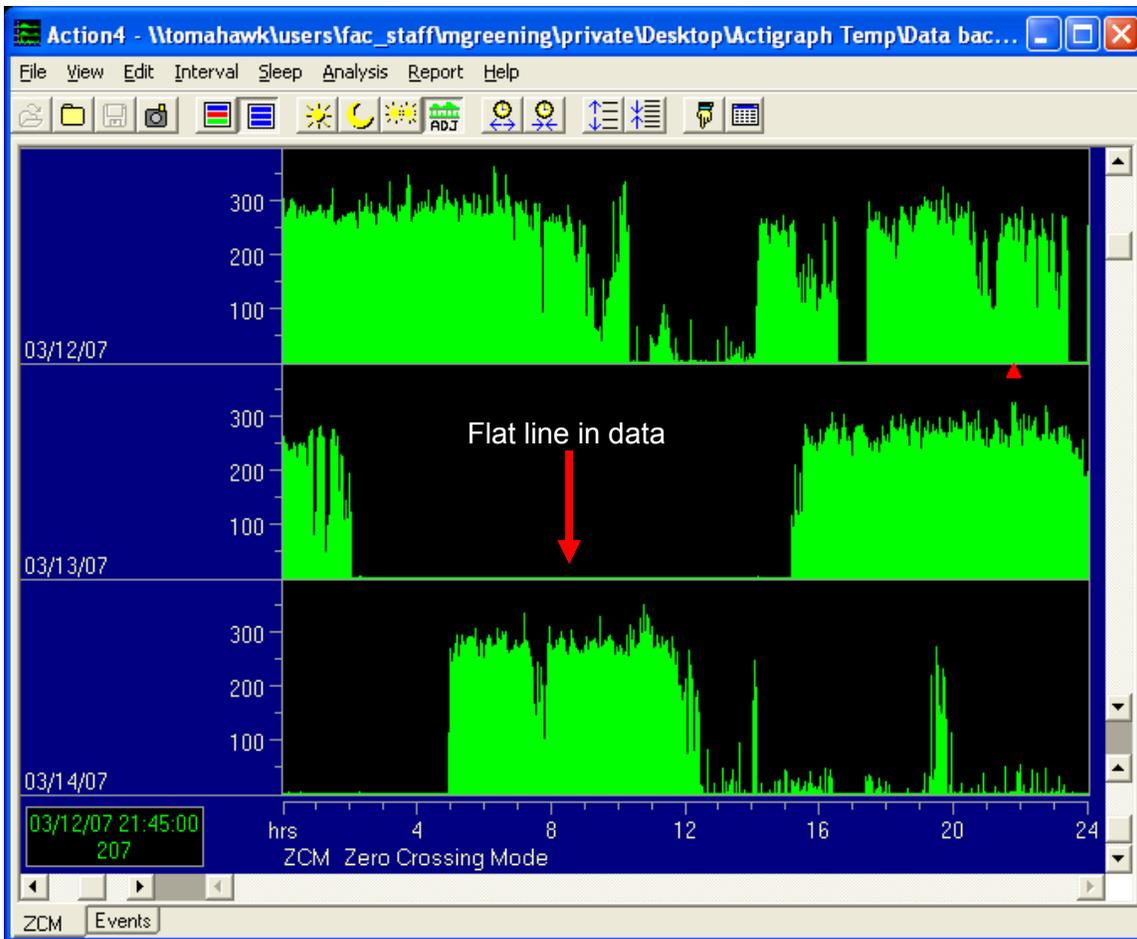
**Figure 11. Action4 Software Displaying Collected Motion Logger Data from an Actigraph Device; Flat Line Indicated Device was Removed**
