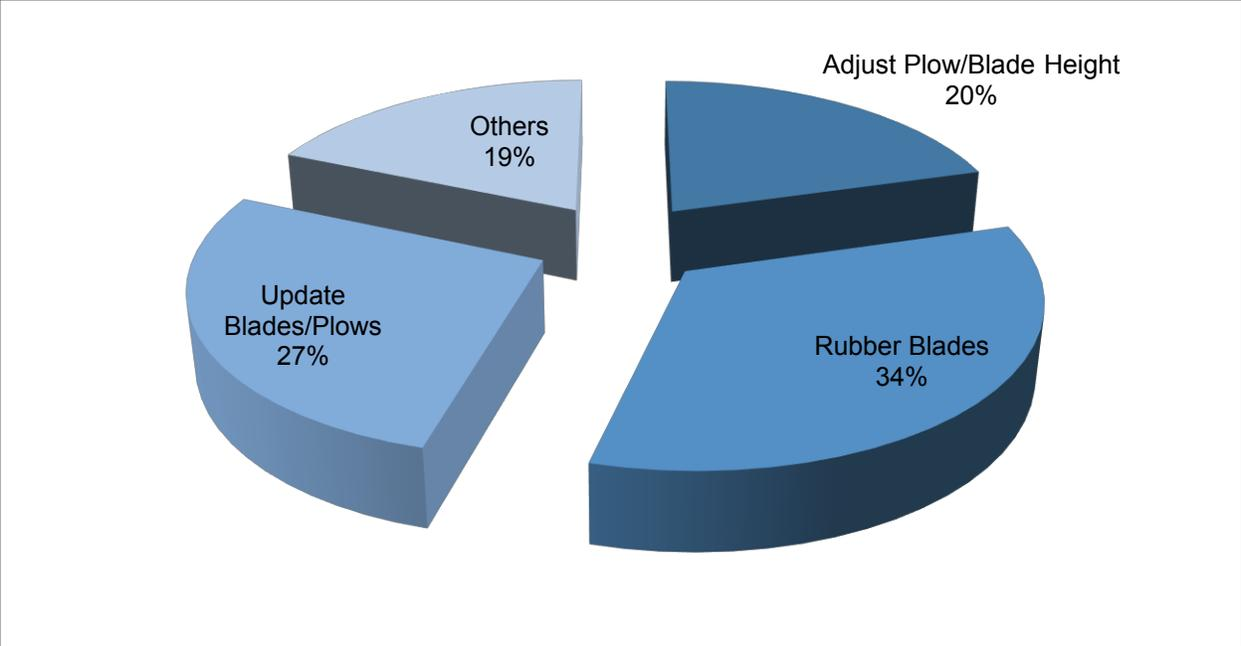
**Figure 78. Best Plow-related Ways to Reduce/Eliminate Vibration Sources**
