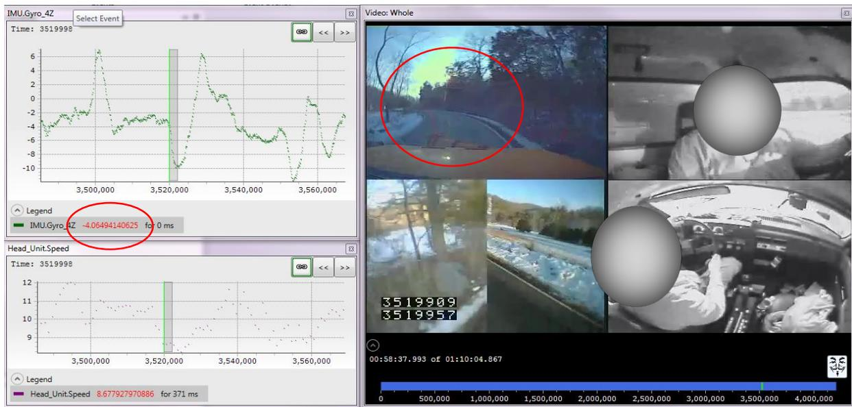
**Figure 14. Example of a Non-conflict Event (with a Valid Trigger) where the Driver's Swerve (Quick Steering) was -4.065 (trigger was set to 12.0 g)**
