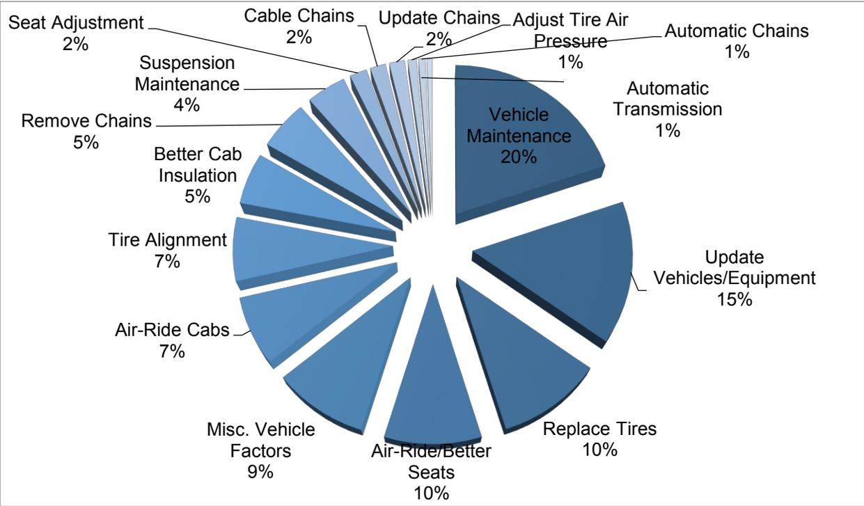
**Figure 77. Best Vehicle-related Ways to Reduce/Eliminate Vibration Sources**
