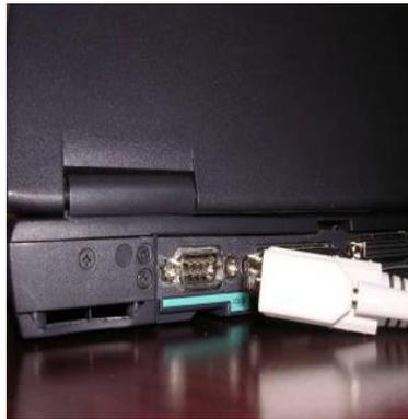
**Figure 49. Serial Port on Computer Back**
