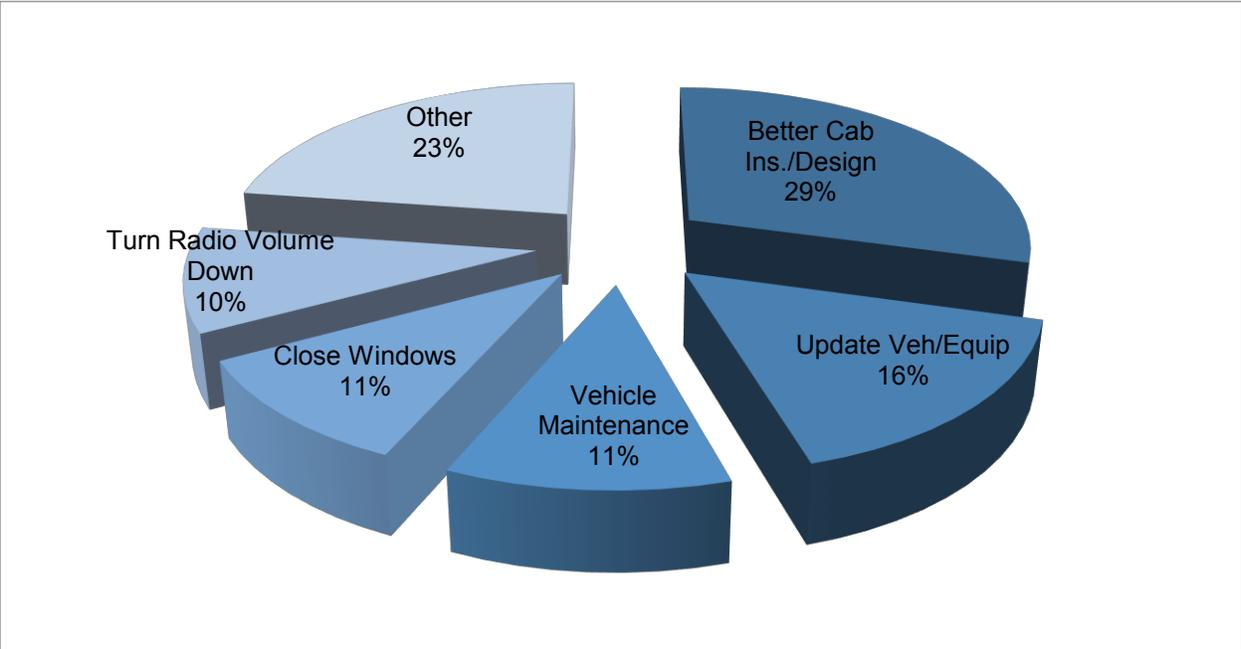
**Figure 85. Best Vehicle-related Methods to Reduce/Eliminate Noise**
