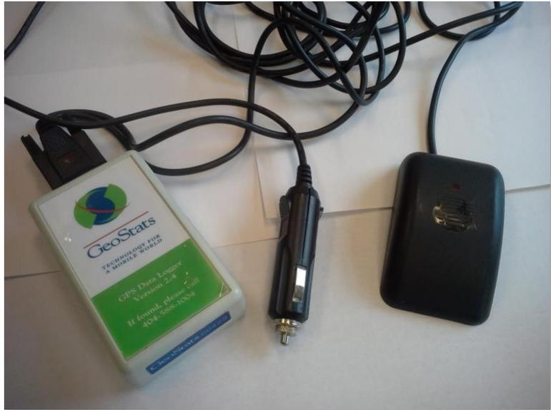
**Figure 7** GeoStats GeoLogger (l. to r.) datalogger, 12V adapter, and antenna
