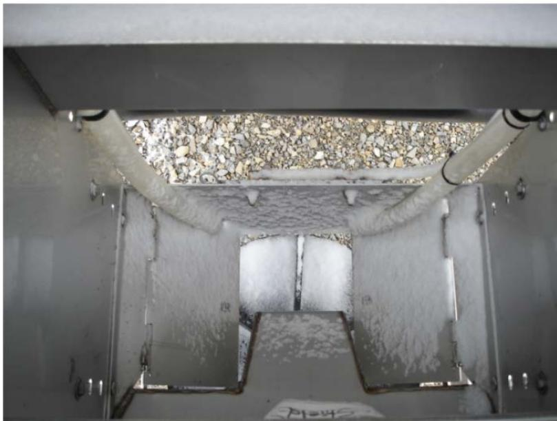
Figure 8: Spray nozzles in the spreader chute of a pre-wetting system (Thompson Engineering Company 2014)
