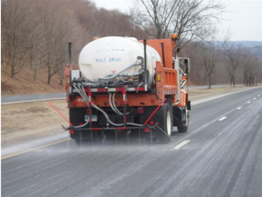
**Figure 4: A typical anti-icing operation on dry pavement (Connecticut DOT)**
