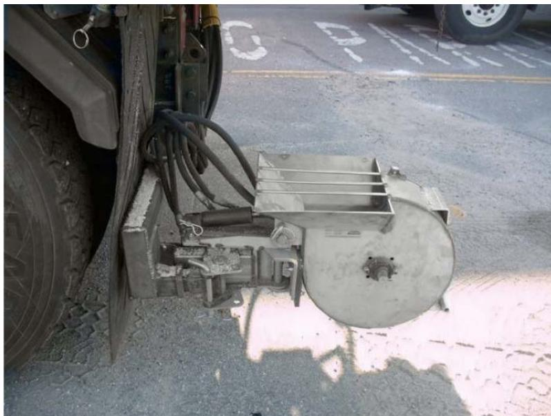
**Figure 9: Zero-velocity spreader equipped on a truck** (Thompson Engineering Company 2014)
