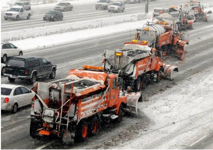
**Figure 5: Snowplows with hopper-type spreaders (right lanes) and “all-liquid” truck (center lane). Photo courtesy of Utah DOT**
