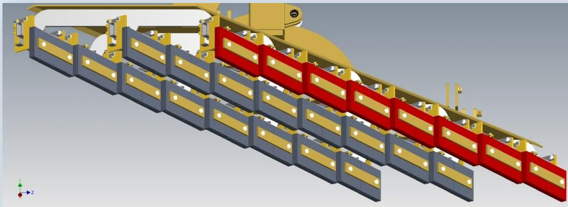
Figure 14. A drawing of the three horizontal and consecutive slush blades developed for testing in Norway. Source: Tellefsdal/AEBI/SCHMIDT
