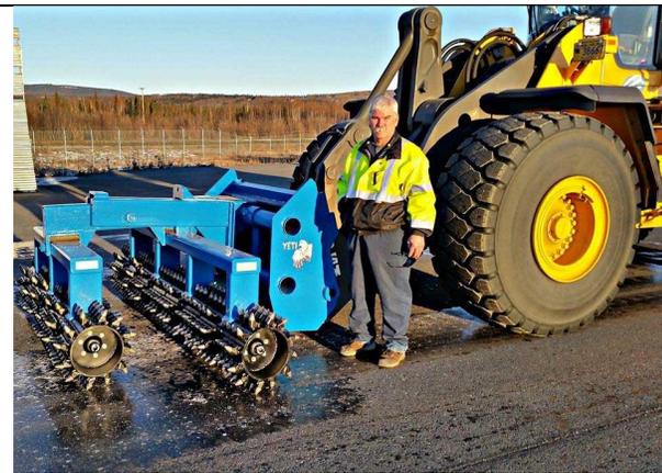
Figure 6. The Yeti icebreaker custom built for use at Fairbank International Airport. Source: [http://dot.alaska.gov/comm/pressbox/arch\\_2015/PR15-2554.shtml#](http://dot.alaska.gov/comm/pressbox/arch_2015/PR15-2554.shtml#) (<https://www.youtube.com/watch?v=XJiWOBvFMil>)
