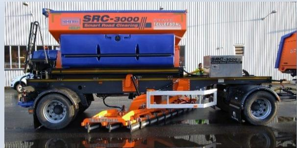
Figure 13. Snowplow vehicles with tow behind trailers with slush blades used by the Norwegian Public Road Administration. Source: Tellefsdal/AEBI/SCHMIDT
