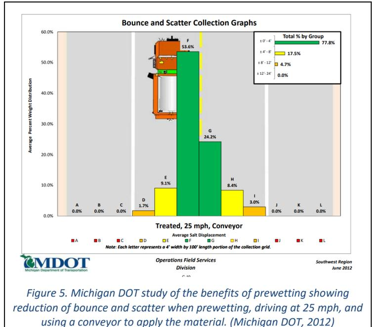
Figure 5. Michigan DOT study of the benefits of prewetting showing reduction of bounce and scatter when prewetting, driving at 25 mph, and using a conveyor to apply the material. (Michigan DOT, 2012)
