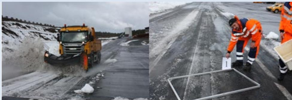
Figure 19. Field test, plowing slush with rubber blades at 40 mph; left before, right after showing data collection. Photos provided NPRA.
