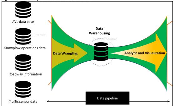
Figure 19- Visual Representation of a Generic Stack
