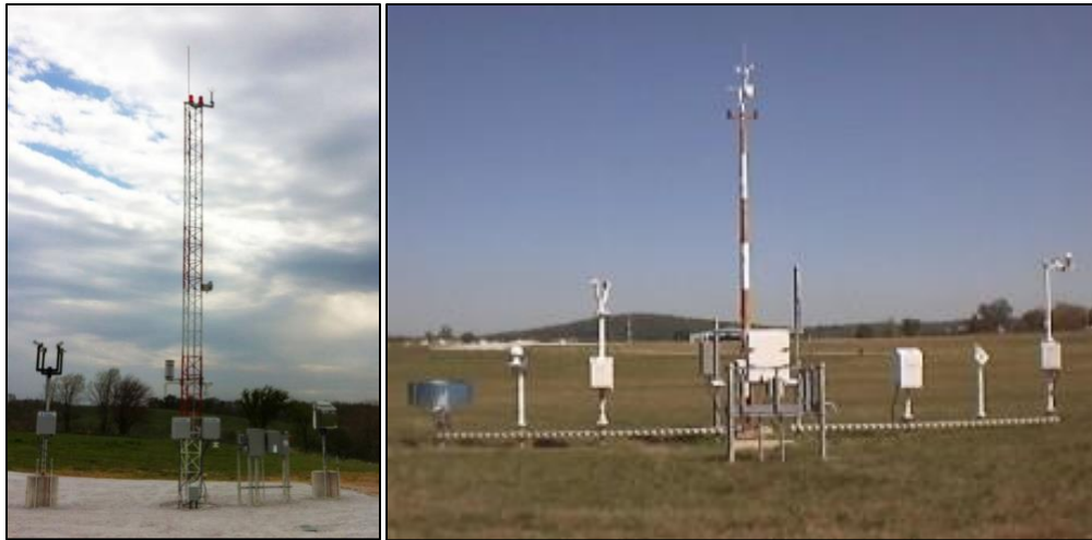
Figure 13: Example images of ASOS (left) and AWOS (right). Image source: https://www.allweatherinc.com/programs/ .
