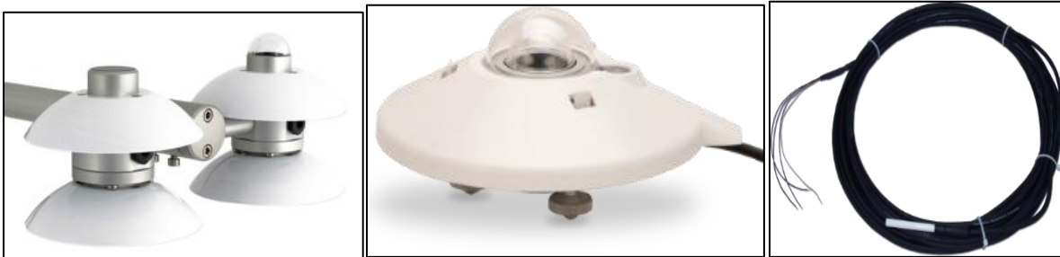
Figure 11: At left, a net radiometer, which includes two pyranometers (to detect incoming and outgoing shortwave radiation) and two pyrgeometers (to detect incoming and outgoing longwave radiation). At center, a pyranometer. At right, a temperature probe with cable.
