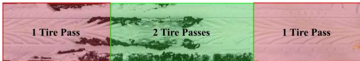
Figure 5. Pavement sample with trafficked snow showing where one tire (red) versus two tires (green) traffic the sample.
