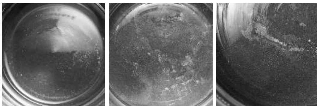
Figure 43. Salt precipitation out of solution E (left to right: E1, E2, E3) at 15°F.
