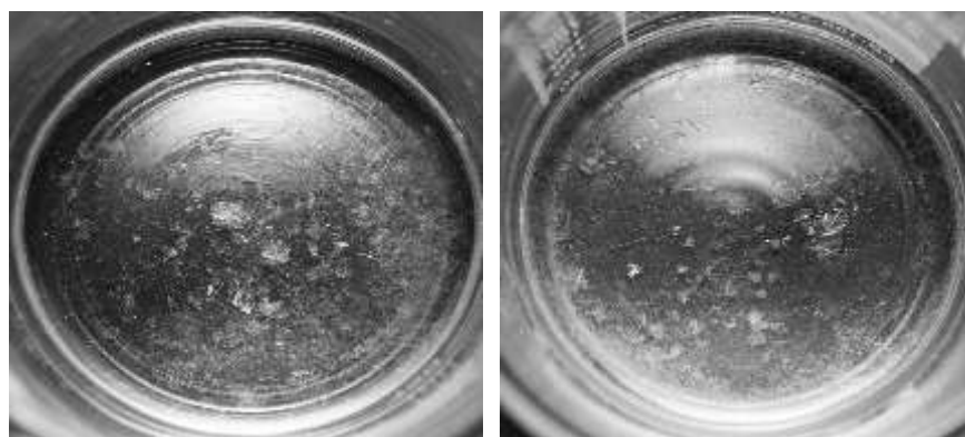
Figure 60. Ice crystal formation and salt precipitation in solution D2 (left) and D3 (right) at -6°F.
