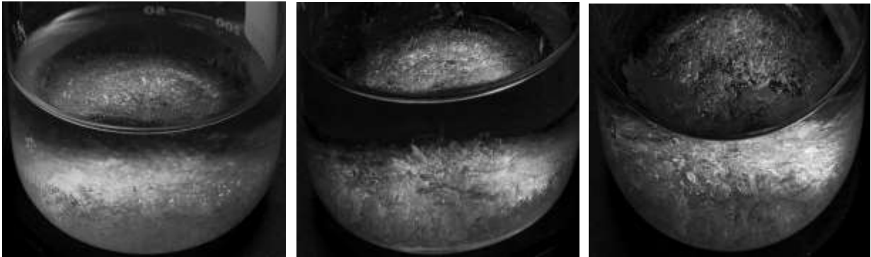
Significant ice crystal formation and minor salt precipitation at 0°F for G triplicates (1 to 3: L to R)
