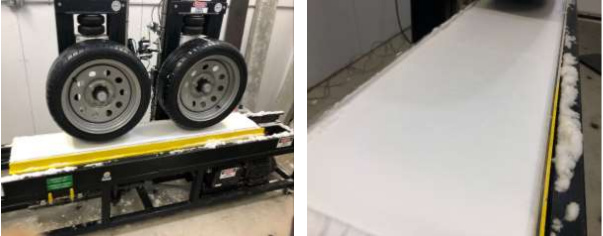
Figure 4. Trafficking machine in the Sub-Zero Research Lab showing (left) the tires lifted above the compacted snow sample and (right) and close up of the compacted snow sample.
