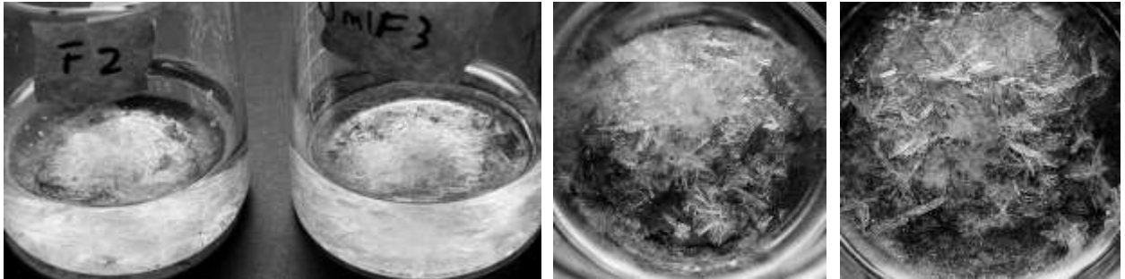
Significant ice crystal formation and salt precipitation for solution F2 and F3 (left), close-up images of F2 (middle) and F3 (right) at -6^{\circ}\text{F}
