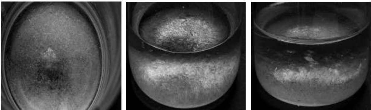
Significant ice crystal formation and minor salt precipitation at 0°F for H triplicates (1 to 3: L to R)
