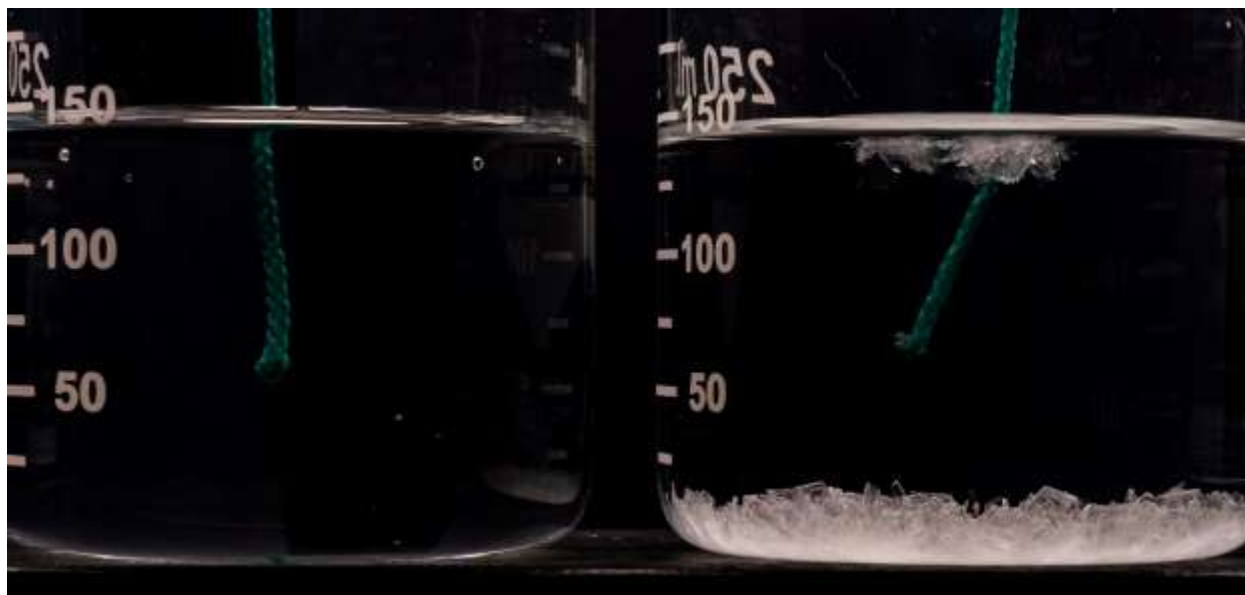
Figure 68. Ice crystal growth, salt precipitation, and potentially dihydrate salt formation in the 27 wt.% NaCl solution (right) compared with 23.3 wt.% NaCl solution with no ice crystal growth or salt precipitation at 5°F. Note that the string was added to serve as a nucleation point.
