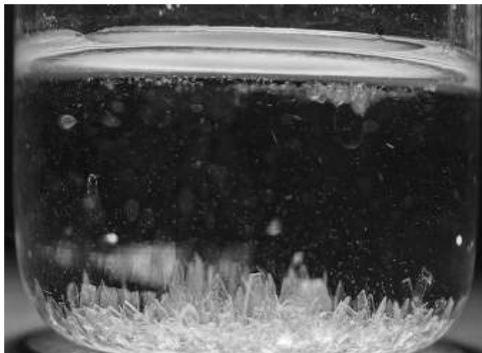
Figure 66. Brine solution showing crystals suspended in the brine solution and salt precipitated out at the bottom of the beaker. Test conditions: -6°F, solution H (28 wt.% NaCl).
