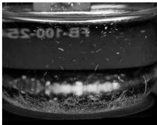
Figure 67. Brine solution showing both ice crystals suspended in the brine solution and salt precipitated out at the bottom of the beaker. Test conditions: 0°F, solution E (25 wt.% NaCl).
