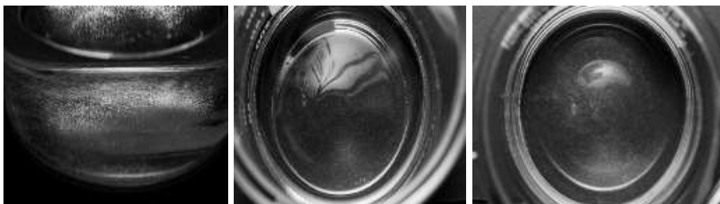
Figure 57. Minor salt precipitation from solution D1-3 (left to right) at 0°F. No visible ice crystal formation.
