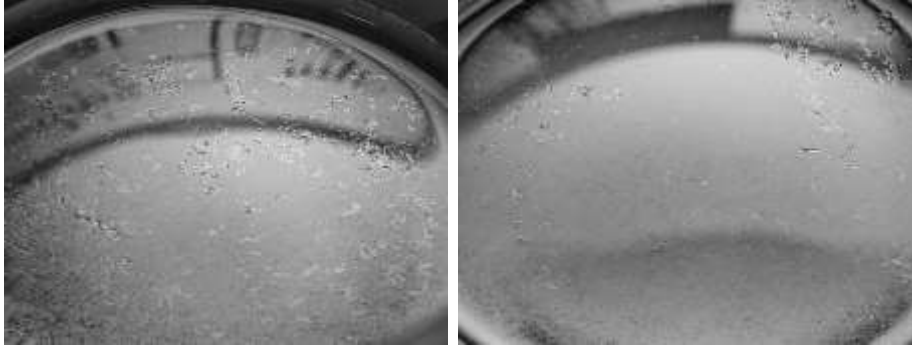
Figure 32. Ice crystal formation in beakers G2 (left) and G3 (right) at 32°F.
