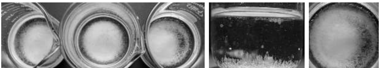
Significant ice crystal formation and salt precipitation for solution H triplicates (left), H2 (middle), and H3 (right) at -6^{\circ}\text{F}
