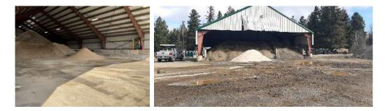
Figure 7.4. Measuring the Washington State DOT pile before and after a small volume is removed.
