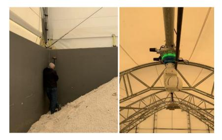
Figure 6.5. Measuring the Salt Shed with the Carlson BRx7 GPS receiver and RT4 Data collector.
