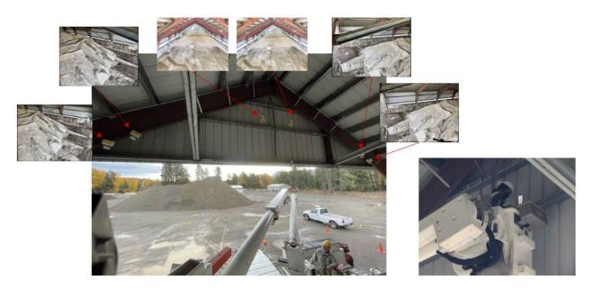
Figure 6.3. Bullfrog facility with three camera pairs at the loading end of the shed.
