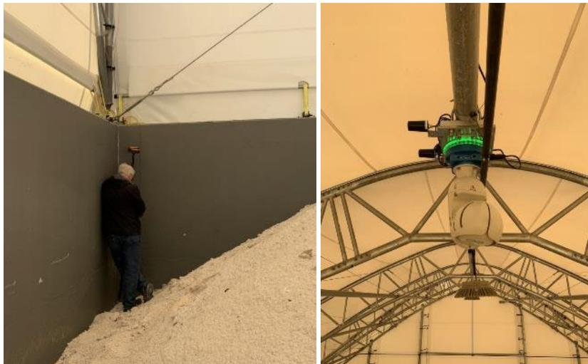
**Figure 6.5.** Measuring the Salt Shed with the Carlson BRx7 GPS receiver and RT4 Data collector.
