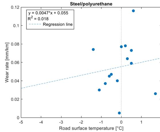
Figure D-0-13: Scatterplot of the wear rate versus the road surface temperature
