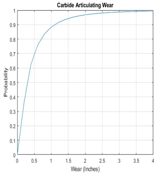
**Figure 5-13: Carbide Articulating Wear Cumulative Distribution**
