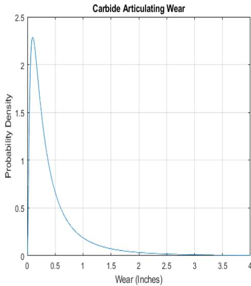
**Figure 5-12: Carbide Articulating Wear Probability Density Distribution**
