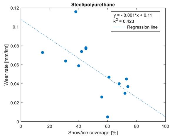
**Figure 4-16: Correlation of Wear Rate and Snow/Ice Coverage for Steel/Polyurethane Blades**
