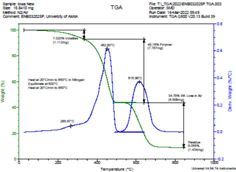
Figure 4-37: TGA Thermogram Obtained on the Iowa Polymer Component
