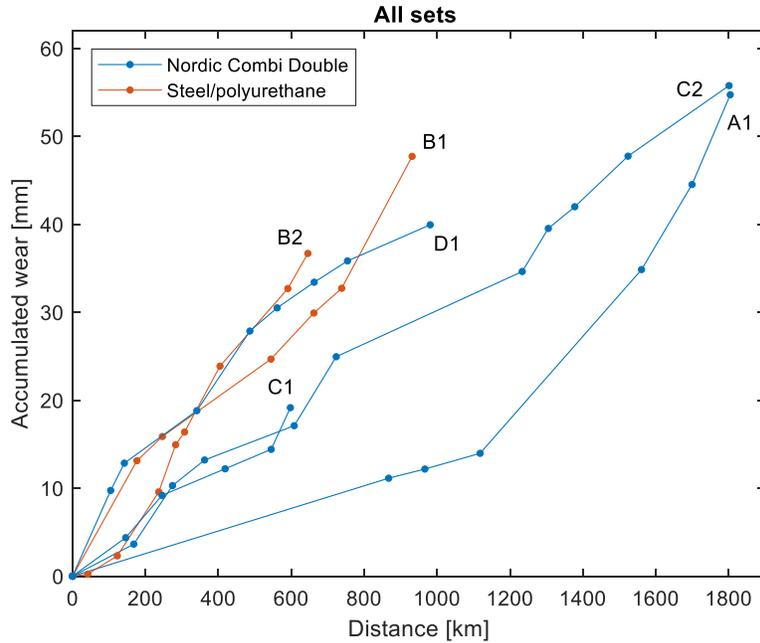
**Figure 4-14: Accumulated Wear as a Function of Plowing Distance**
