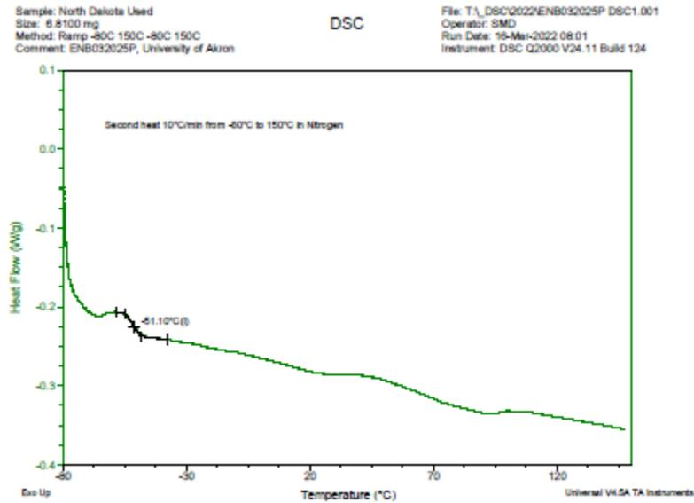
Figure 4-32: DSC thermogram Obtained on the North Dakota – Used Polymer Component During the Second Heating Cycle
