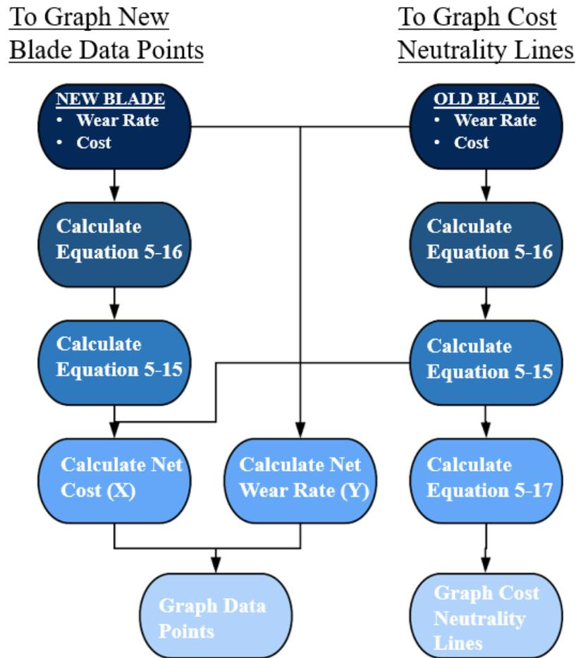
**Figure 5-18: Calculating Diagram**
