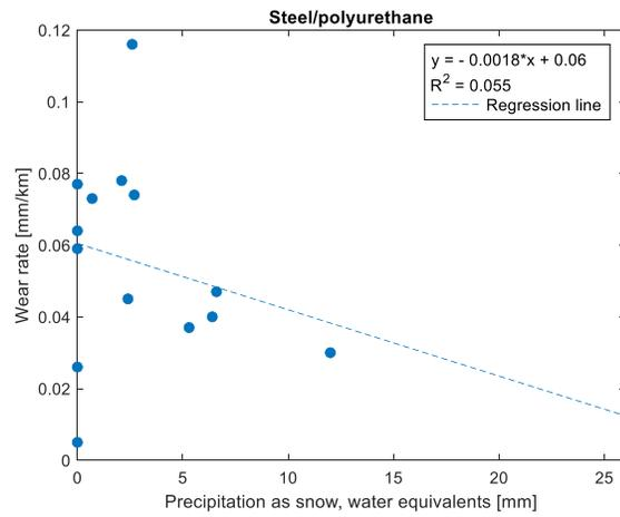
Figure D-0-12: Scatterplot of the wear rate versus the amount of fallen snow (in mm water equivalent)
