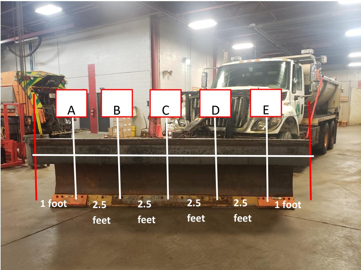
**Figure C-0-1: Location of measurements along a 12-foot blade**
