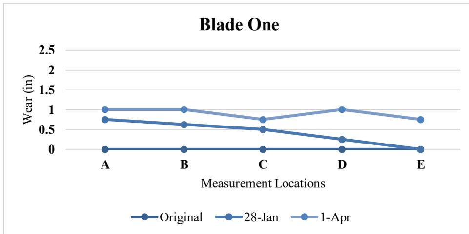
**Figure 4-5: Blade One Tested in Moscow/Potlatch**
