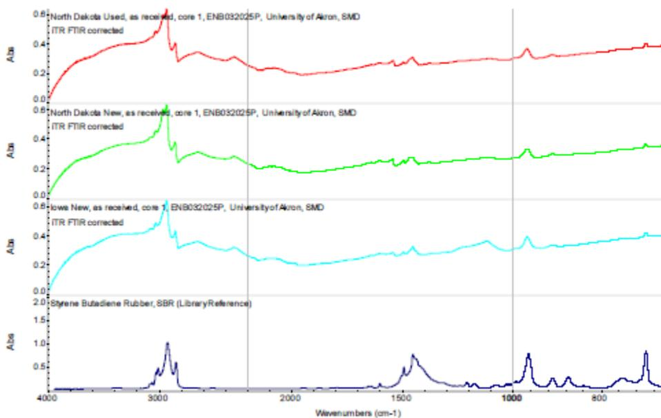
Figure 4-29: FITR Spectra Obtained on the Polymer Component of the Blades as Received.
