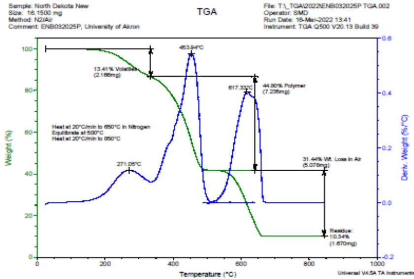
Figure 4-35: TGA Thermogram Obtained on the North Dakota – New Polymer Component
