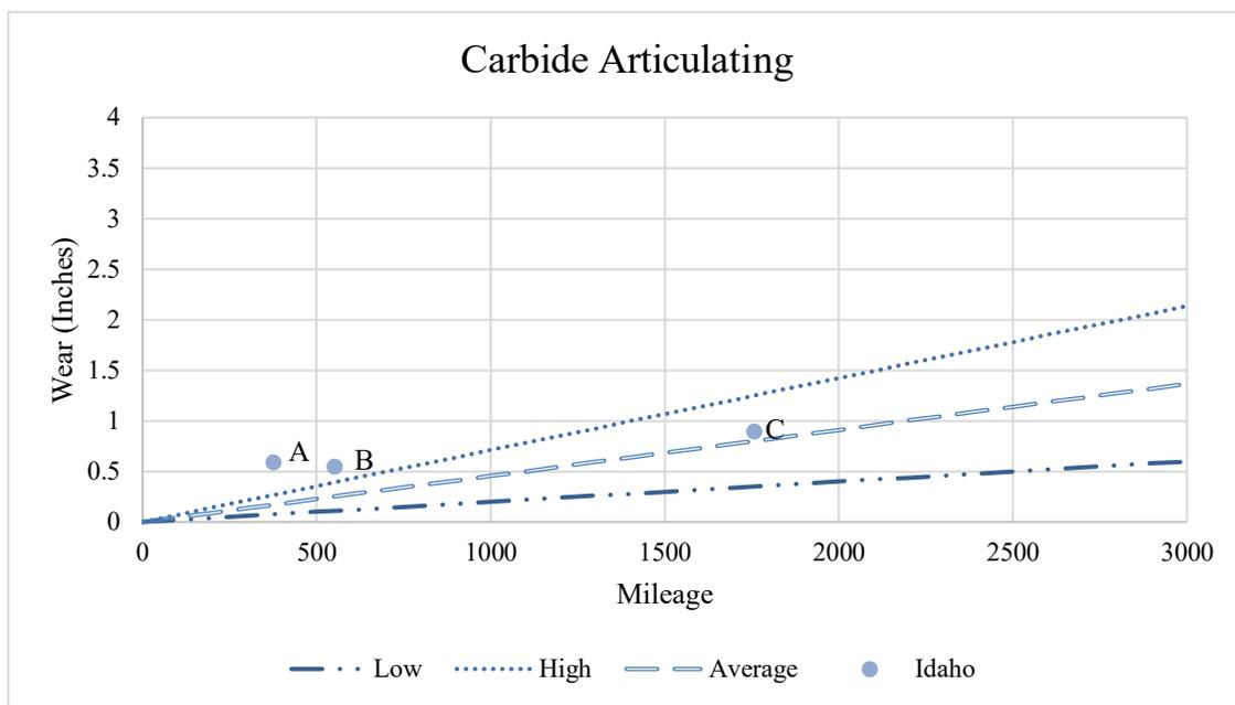
**Figure 5-4: Carbide Articulating Blade**
