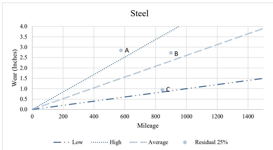
Figure 5-5: Steel Blade
