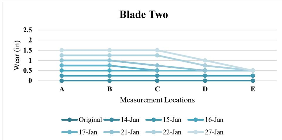
**Figure 4-6: Blade Two tested in Soda Springs**
