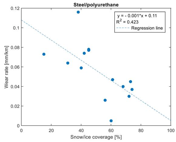
Figure D-0-16: Scatterplot of the wear rate versus the snow/ice coverage
