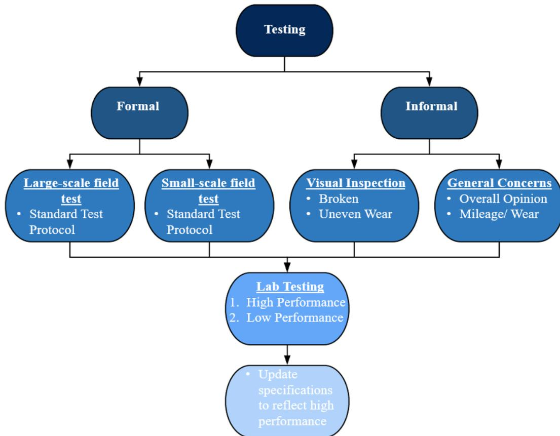
**Figure 4-39: Integration of Field and Lab**
