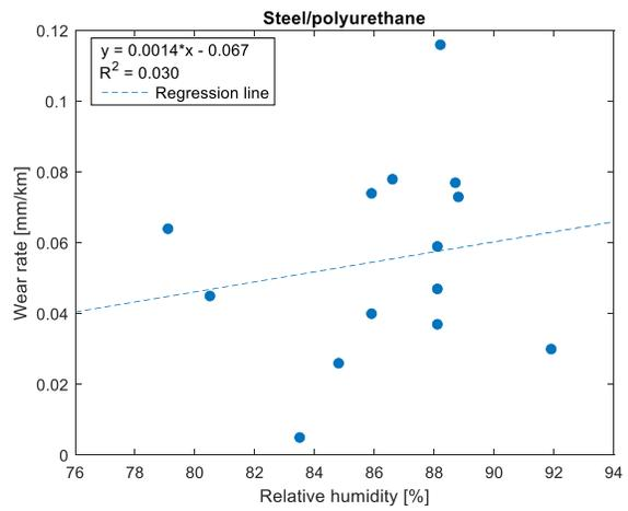
Figure D-0-15: Scatterplot of the wear rate versus the relative humidity
