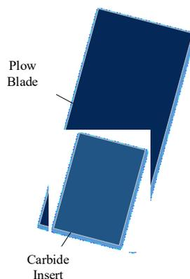
**Figure 2-8: Carbide Insert**
