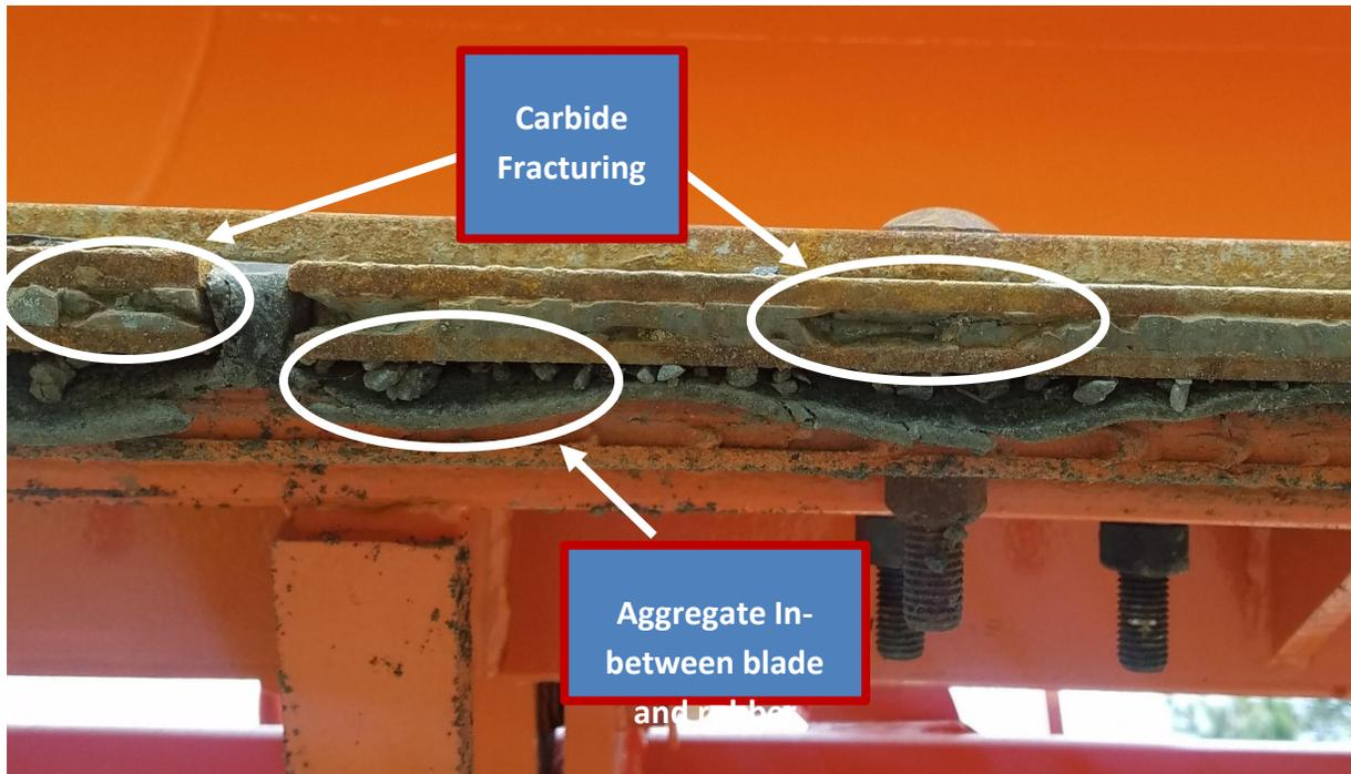
**Figure 4-9: Blade Failure in Idaho Case Study**
