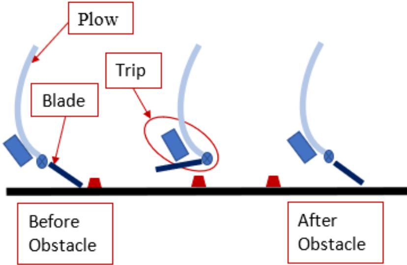
Figure 2-4: Tripping Mechanism
