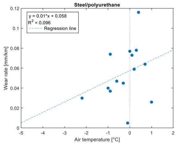
Figure D-0-14: Scatterplot of the wear rate versus the air temperature
