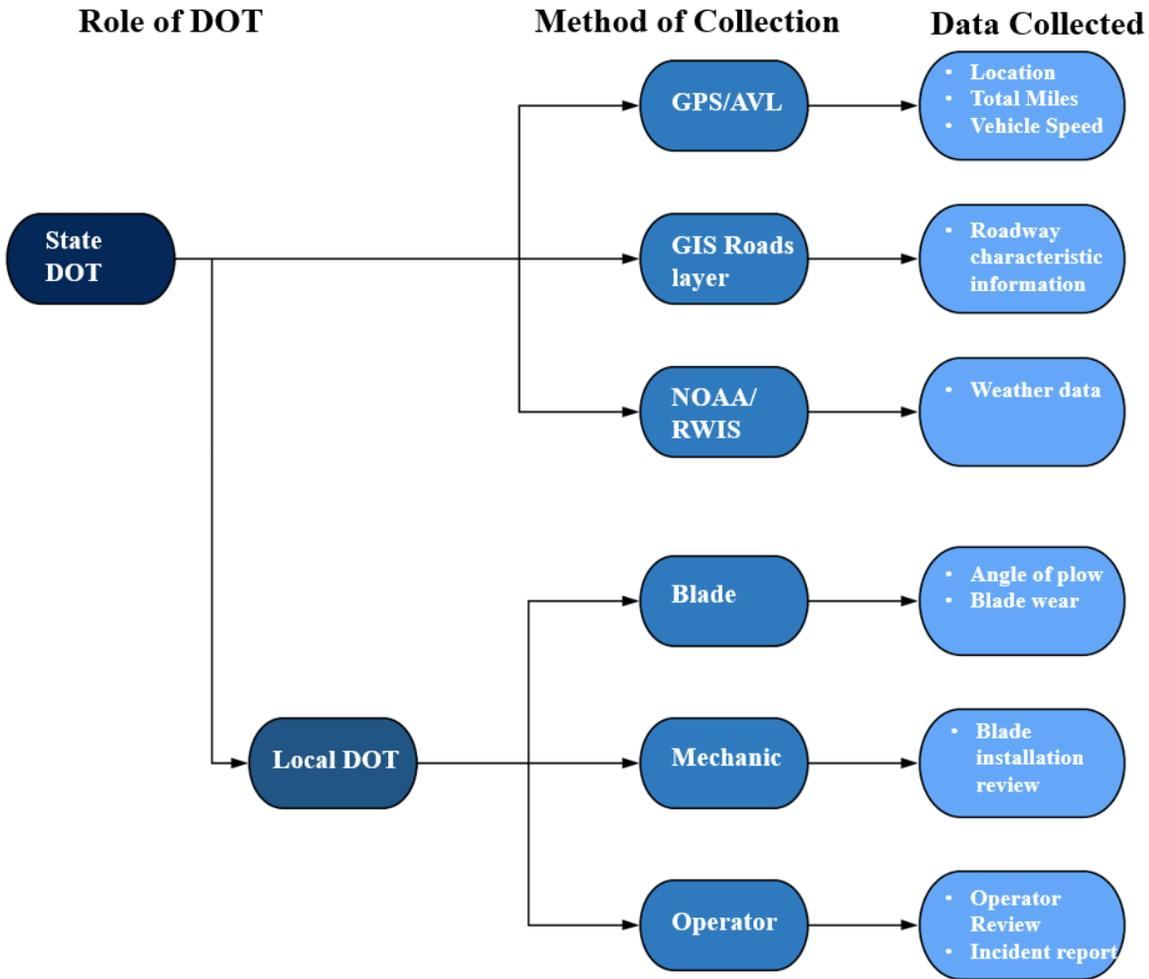
Figure 4-1: Blade Testing Protocol
