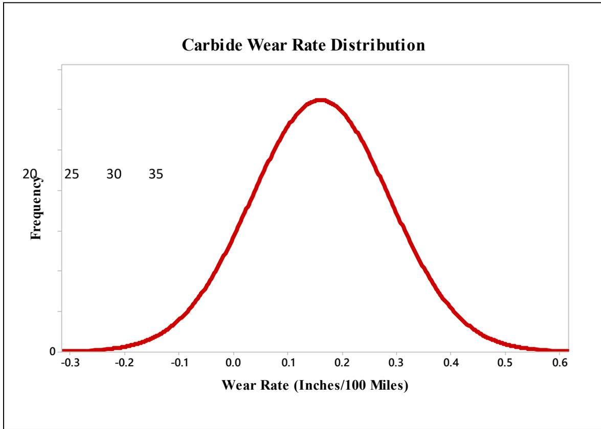
Figure 5-2: Carbide Wear Histogram
