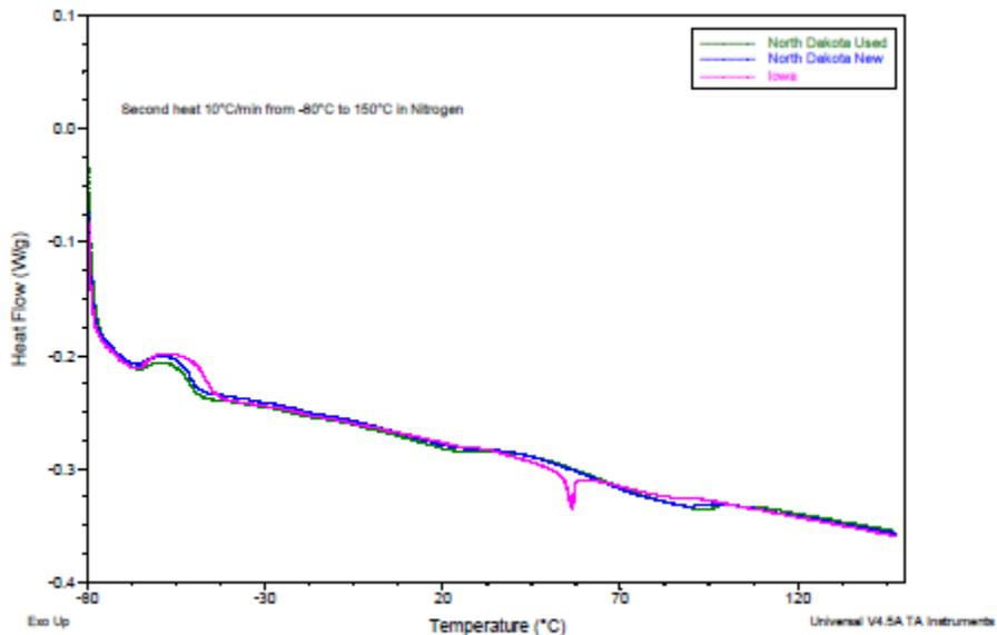
Figure 4-34: Overlay of the DSC Thermograms Obtained on the Three Polymer Components During the Second Heating Cycle
