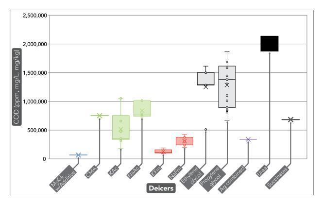
Figure 4. Graphical display of COD values reported in the literatures and shown in Tables 18-23 with units converted to be consistent for comparison.
