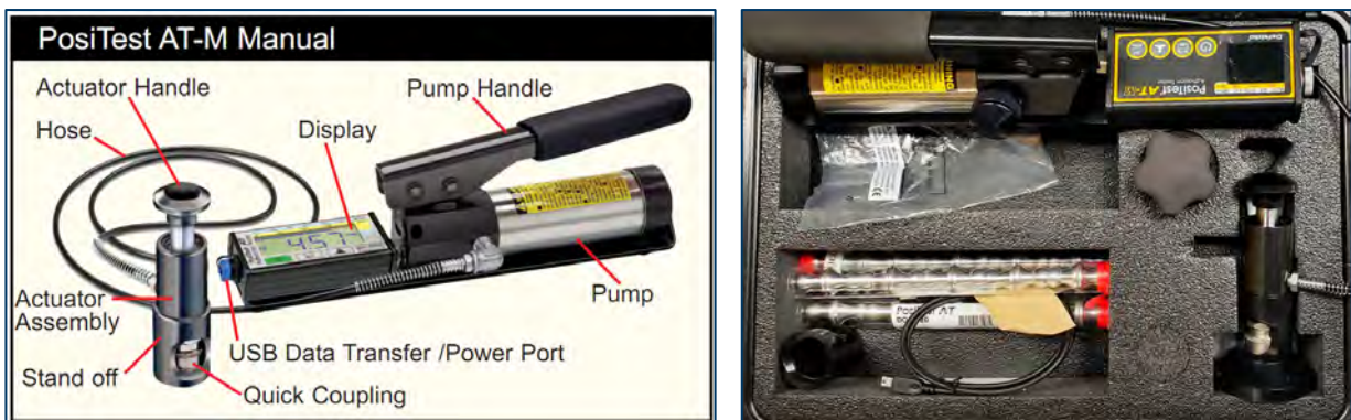
Figure 2.11 PosiTest® AT-M pull-off adhesion tester to conduct ASTM D4541 ( Instruction Manuals / DeFelsko, n.d. )
