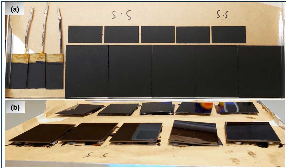
Figure C 3 Paint highlights: (a) Armour Seal dried (b) drying set up for Lubra Seal salt spray coupons
