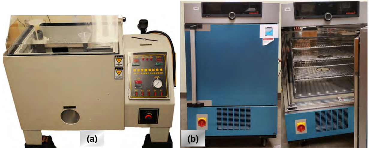
Figure 2.8 Equipment used to conduct SAE J2334 (a) Salt spray chamber, 110L capacity (110V) (b) Humidity chamber (Memmert, USA, LLC®) for humid and dry cycles
