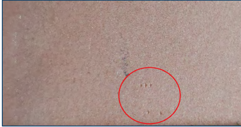
Figure 2.14 Micro indentations made on the S-AP coupon, after the Vickers hardness testing
