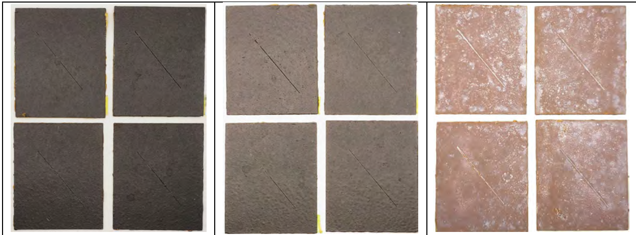
Figure C 24 Coupons for SAEJ2334 (cyclic salt spray test) – Day 60 (left to right) Al-AS, SS-AS, and S-AP
