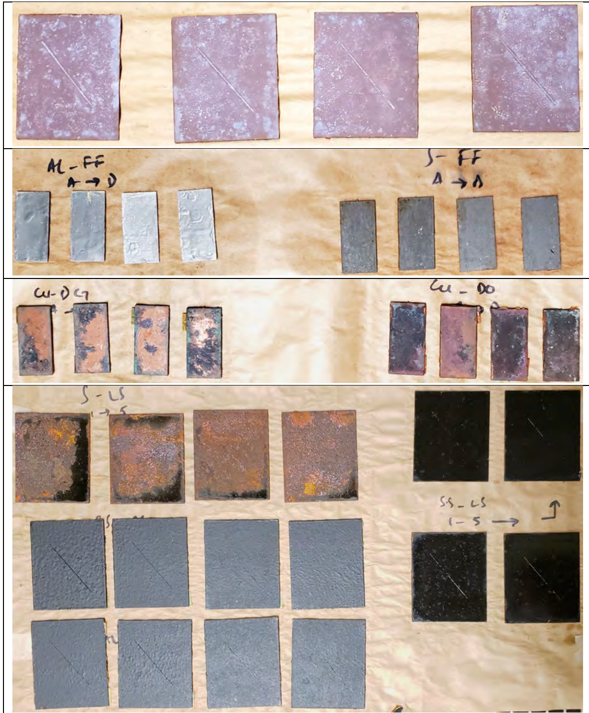
Figure C 15 Coupons for SAEJ2334 (cyclic salt spray test) – Day 60 (a) S-AP (b) Al-FF (left) and S-FF (right), (c) Cu-DG (left) and Cu-DO (right), (d) remaining scribed coupons (S-LS, SS-LS, SS-AS, Al-AS)
