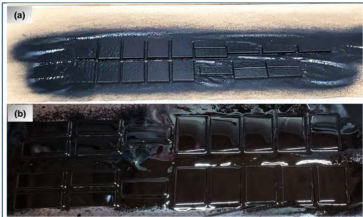
Figure C 2 Paint shop highlights: (a) Armour Seal and (b) Lubra Seal, both applied using pistol grip spray gun
