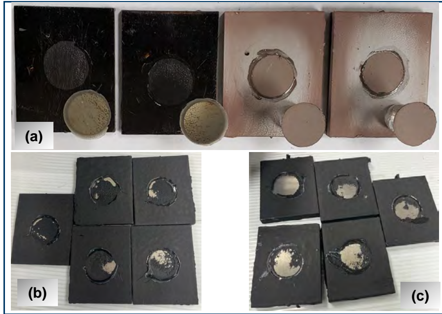
Figure 2.12 Coupons used in pull-off adhesion test: (a) S-LS (black coupons) and S-AP coupons (dark pink), (b) SS-AS, and (c) Al-AS
