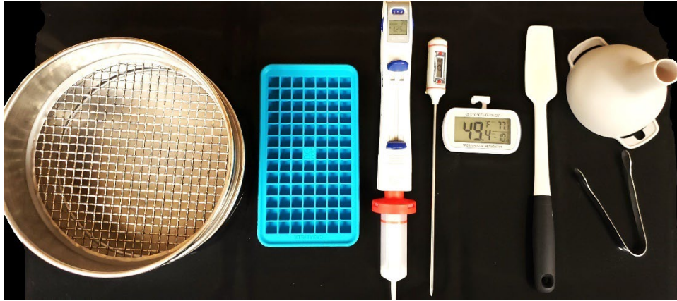
Figure 5. Items used in modified IMCRT (left to right): a #4 sieve (1/4" mesh opening), a mini-ice cube tray made by Casa Bella®, an Eppendorf® repeater pipette M4, a stem thermometer (only for liquid samples), a digital thermometer for freezers, a silicon spatula, a plastic funnel, and a pair of stainless tongs.
