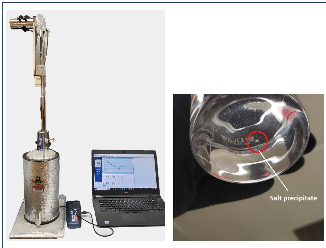
Figure 29. Linear agitation, ice bath, and data logger setup for FPT (left); salt precipitates in a 24 wt. % solid control solution at 13.4°C (right)
