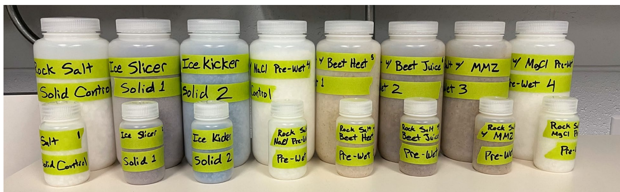
Figure 2. Samples made for testing following gradation analysis and prewetting. Small bottles remained at WTI for testing, larger bottles were sent to WSU for testing.
