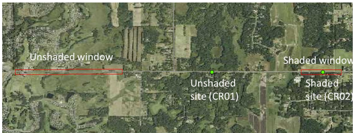
Figure 14: Satellite photo of the unshaded and shaded windows (red squares) used to identify truck temperature data for comparison to the radiometer measurements (green circles).
