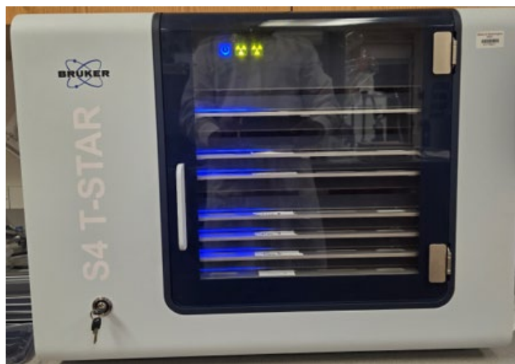
Figure 10. Elemental analysis using a Bruker S4-TSTAR XRF device
