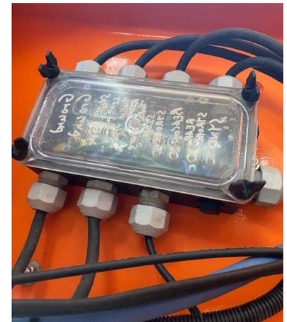
Figure 13. Junction Box in Tow Plow
