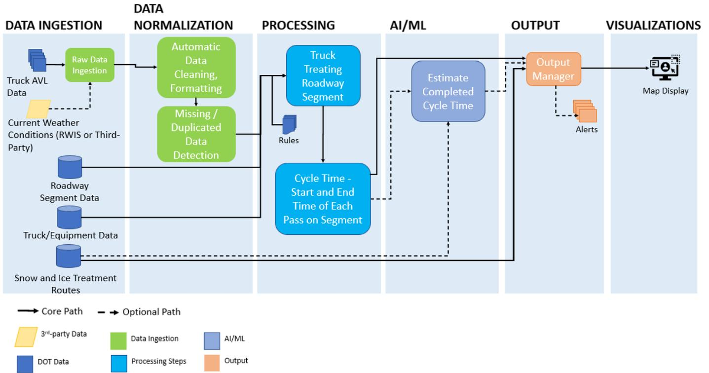
Figure 1: High-level Architecture of Cycle Time Tool
