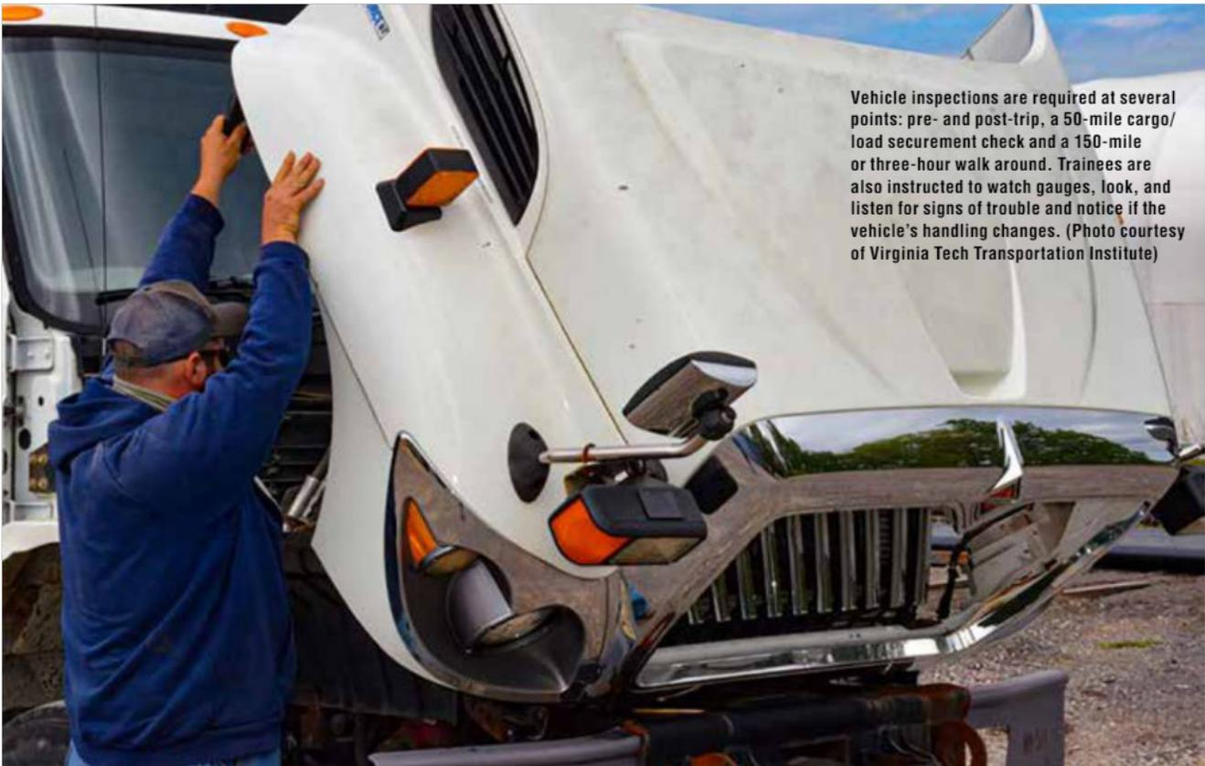
Vehicle inspections are required at several points: pre- and post-trip, a 50-mile cargo/load securement check and a 150-mile or three-hour walk around. Trainees are also instructed to watch gauges, look, and listen for signs of trouble and notice if the vehicle's handling changes. (Photo courtesy of Virginia Tech Transportation Institute)
