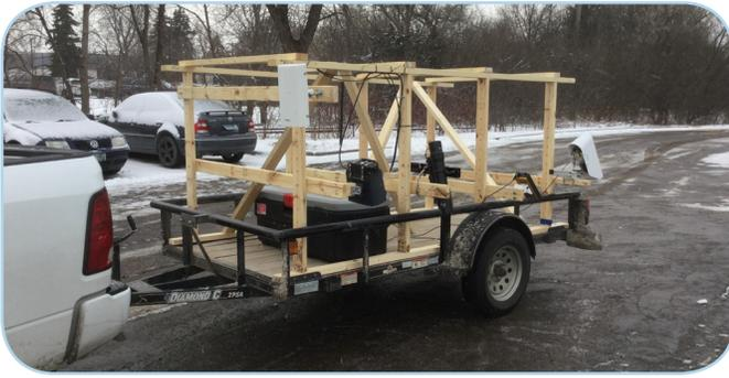
Researchers built an adjustable rig onto a trailer to allow all four mobile sensors to be tested simultaneously, each at its optimum mounting height. The rig was used in live traffic as well as closed-course testing.
