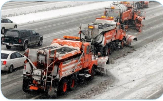
Common equipment for winter road maintenance includes snowplows with hopper-type spreaders (lower left) and trucks that hold tanks of liquid deicers (upper right). Photo courtesy of Utah DOT.
