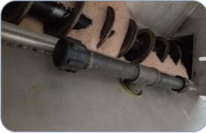
A screw conveyor mounted inside a truck pre-wets dry salt before it's applied to the road. (Photo courtesy of North Dakota DOT.)
