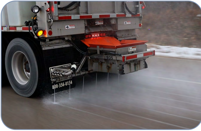
Treating roads by directly applying salt brine provides similar performance results compared to traditional granular salt but uses significantly less salt.
