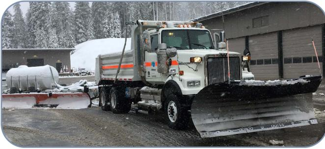
This Tow Plow has a 22-foot snow clearing path, about twice as wide as that of a standard front plow. Some Tow Plows are bidirectional, providing additional options for clearing the roads. (Photo courtesy of Caltrans.)
