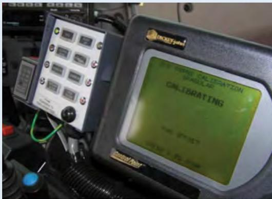
A ground-speed controller in calibration mode.
