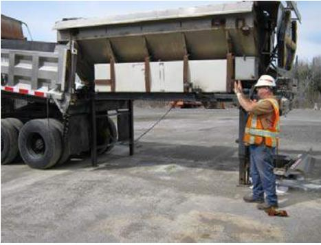
12) The operator will continue to pull forward until the hopper is positioned to allow the front legs of the hopper stand to drop. The spotter will direct the operator to stop and secure the vehicle by putting the vehicle in neutral and applying the parking brake.
