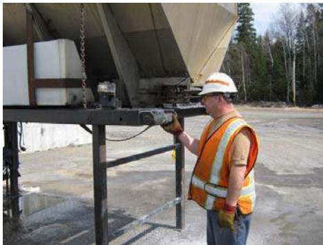
➤ The hopper stand will be inspected for cracks, cracked welds, bent legs and pins, excessive corrosion or other deficiencies that can potentially cause the hopper stand to fail.
