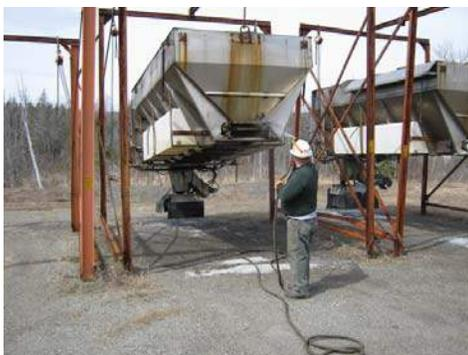
15) Whenever possible, the hopper should be completely washed after removal. **Note: Wear all appropriate PPE.**
