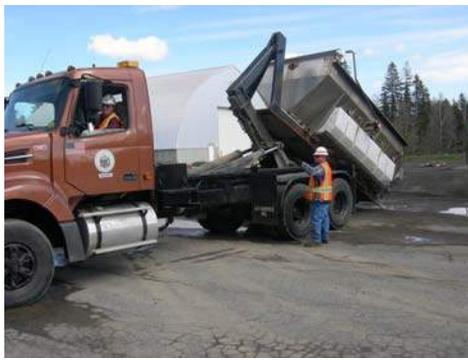
14) As the back of the hopper frame touches the ground, the spotter will direct the operator to release the parking brake. This will cause the truck to be pushed forward as the hopper is lowered.
