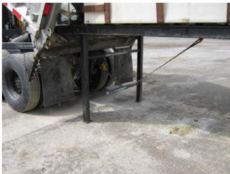
14) The operator will re-enter the vehicle and with the spotter in full view, raise the body until the front legs have contacted the ground. The operator will stop and secure the vehicle.
