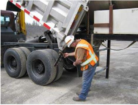
16) To complete the removal process, the spotter will perform a final check to confirm all fittings have been disconnected and then indicate to the operator that it is safe to move the vehicle away from the hopper.
