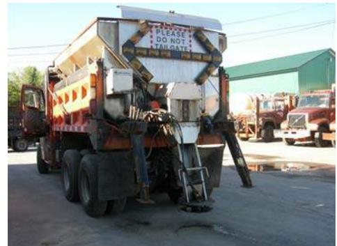
Each of these spreaders is stored using a hopper stand system. The modified spreaders are installed and removed in the same manner as the standard hoppers, while the Stratos system has one additional requirement. The chute/spinner assembly must be raised when removing the spreader. This additional step is documented as step 4A in the [Hopper Removal \(Hopper Stand System\)](#) section.
