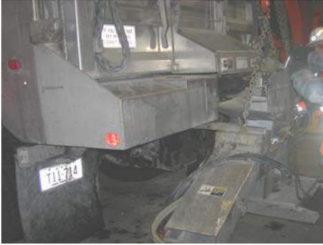
3) The next step is to install the spinner assembly.
