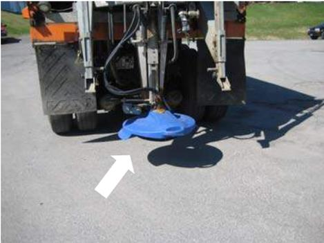
The Schmidt Stratos is designed and used primarily in Europe and it incorporates a specially designed spinner to mix and distribute the treated salt. One additional feature of the Stratos is its ability to spread material in multiple lanes by rotating the spinner opening relative to the road alignment (see picture at left).
