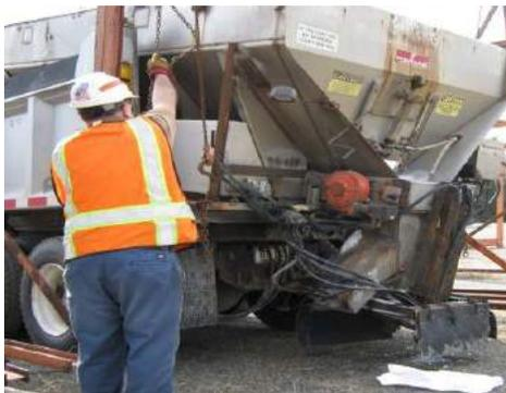
13) The spotter will then raise the hopper using the chain falls, so it clears the truck body by several inches.
