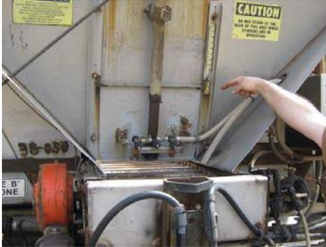
18) Confirm the gate is positioned at the proper gate setting.
