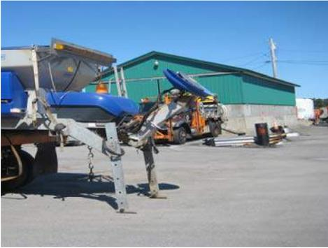
4A) For the Schmidt Stratos Spreader, the chute/spinner assembly must be raised when removing the hopper.
