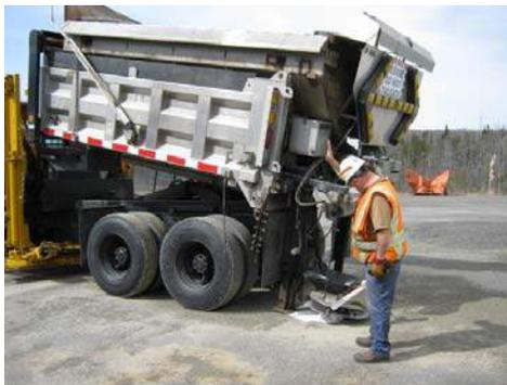
10) The operator will raise the dump body until the rear of the hopper begins to come off the floor of the dump.
