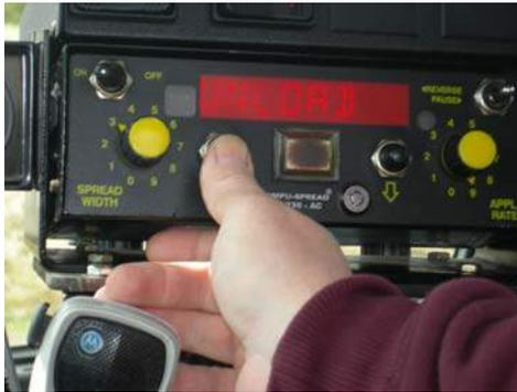
14) Confirm the bed chain or belt is working properly by running the truck in the “unload” mode.
