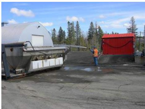
16) To complete the removal process, the hopper should be completely washed. **Note: Wear all appropriate PPE.**
