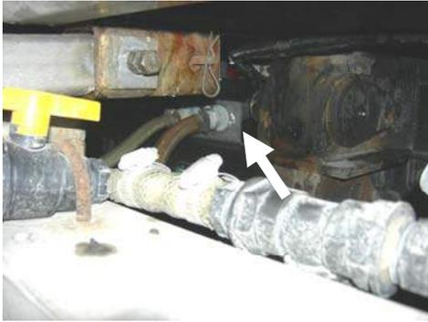
7) To complete the spinner assembly installation, connect the liquid/brine fittings
