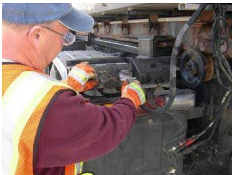
16) To complete the installation process, make one final and overall check of the hopper to confirm all hydraulic fittings and electrical connections are properly attached.
