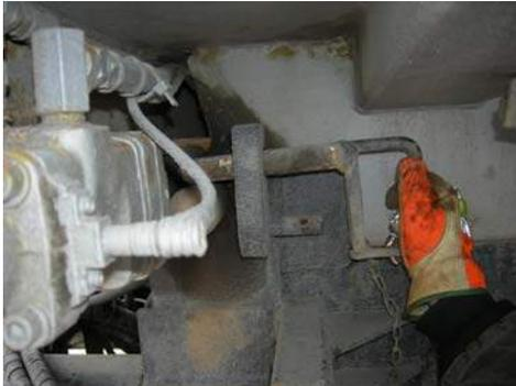
3) Next, remove the pins or locks from the rear hinge point locations and move them to the front locations. **Note: Make certain this process is completed on both sides of the truck body.**
