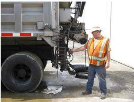
21) To complete the installation process, make one final and overall check of the hopper to confirm safety chains, hydraulic fittings and electrical connections are properly attached.
