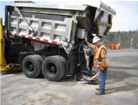
8) With the operator back in the vehicle and the spotter in full view, the operator will raise the dump until the rear legs make contact with the ground and stop the vehicle when directed by the spotter.
