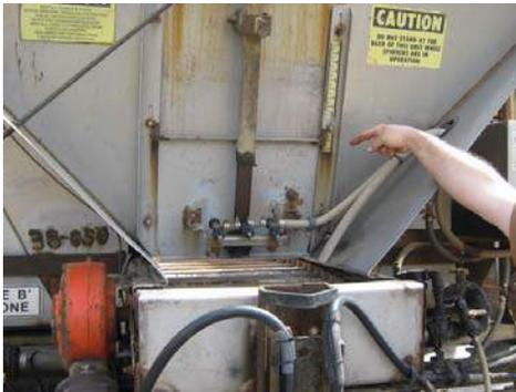
15) Confirm the gate is positioned at the proper gate setting.
