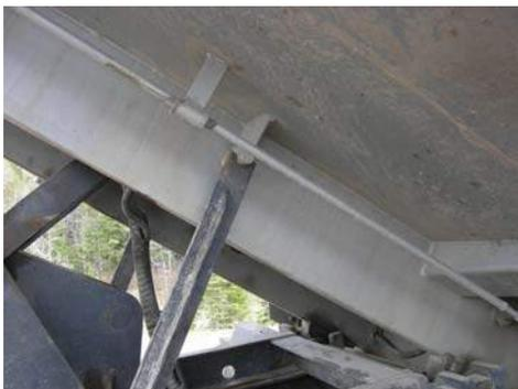
➤ Lift dump body and place dump props into position
