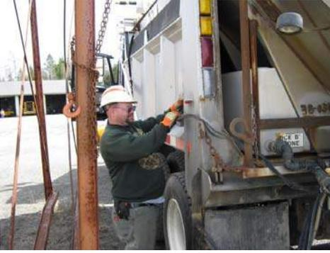
13) Connect all wiring for lighting, controller (Compu-Spread, Cirus, Schmidt), etc. **Note: Check the controller connector to assure a liberal amount of dielectric grease is present.**
