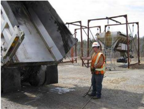
2) During summer use, the body of the truck can become cluttered with gravel, pavement, miscellaneous tools and even an occasional bottle or can. Make certain the body is completely clean of all debris before installing the hopper.
