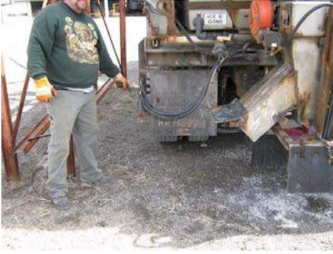
17) Check for hydraulic leaks.
