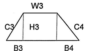
The volume of stockpile between A2 and A3 is  $(A2+A3)/2 \times L2 = (630+690)/2 \times 25 =$
