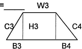
The volume of stockpile between A2 and A3 is  $(A2+A3)/2 \times L2 =$
