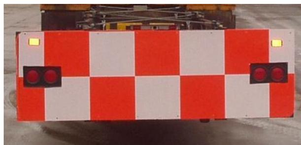
**Figure 2.8 Recommended Checkerboard Marking Pattern (Mid-America Transportation Center)**
