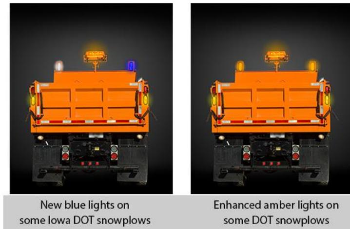
**Figure 2.5 New Rear Lighting on Some Iowa DOT Snowplows**
