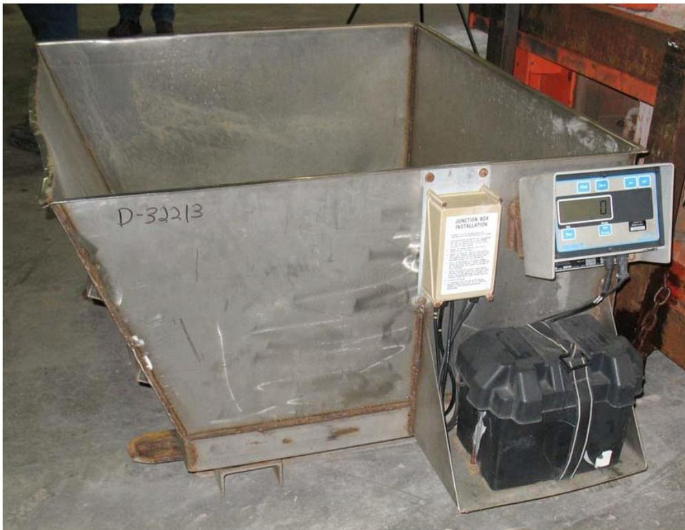
Figure 1. Electronic scale used for calibration
