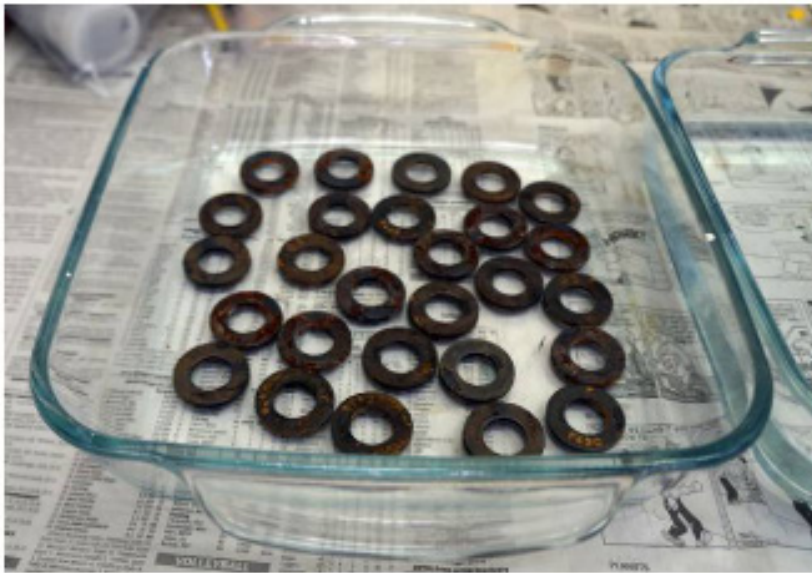
Steel coupons after exposure to product samples in Nebraska DOT's laboratory for corrosion testing.
